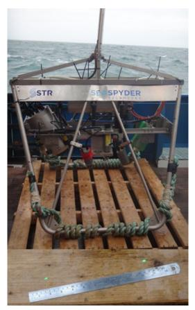
Figure 5. Drop Camera video and still imaging system.
