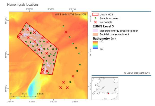
Figure 6. Location of attempted grab stations at Utopia MCZ displaying successful and failed stations.
