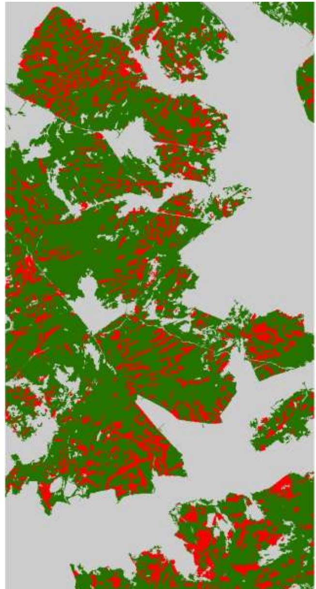
**Figure 1** Example classifications. Phase 1 Development. Vector mapping of 2005 Ikonos imagery of North Yorkshire. Left: raw image; right: image classified using heather mask and extracting one burn class equivalent to Class 1 API or 'new burn'. Note that as with all following images more burns are apparent in the RGB imagery. These are partially revegetated Class 2 burns.
