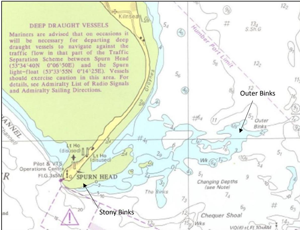
Figure 2 Hydrographic chart of the Spurn area (water depths in metres; chart datum is -3.9m OD; <http://www.ntsif.org/tides/datum>)
