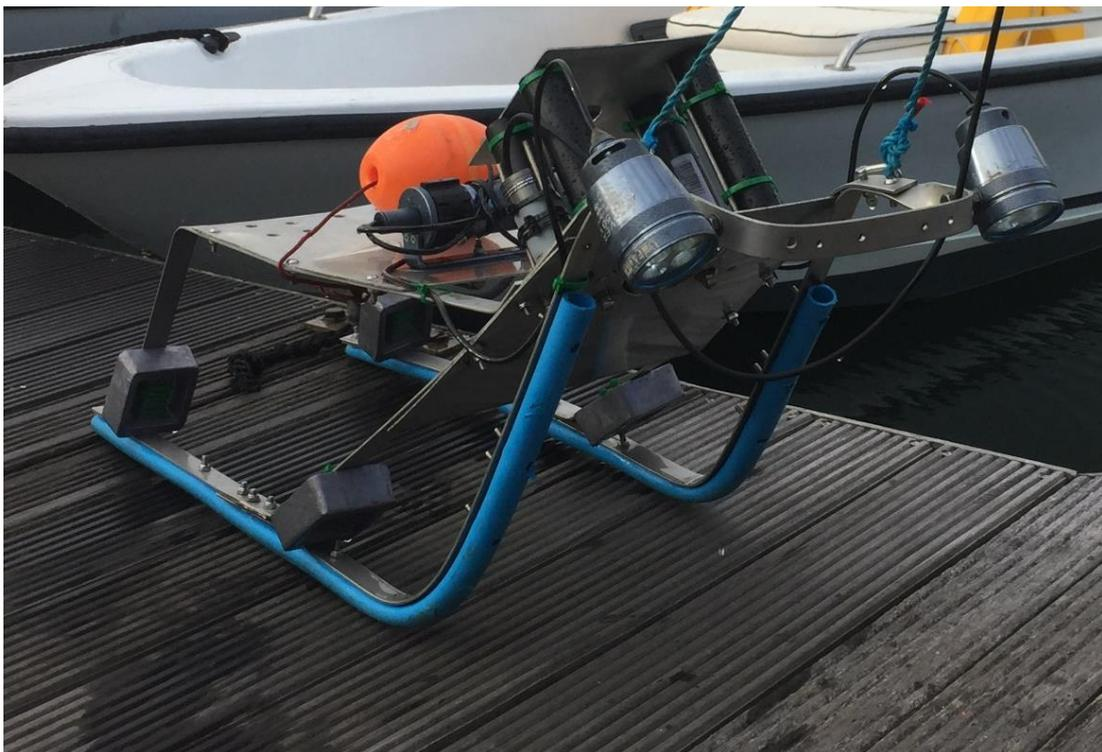
**Plate 1 The camera system used for the video survey**
