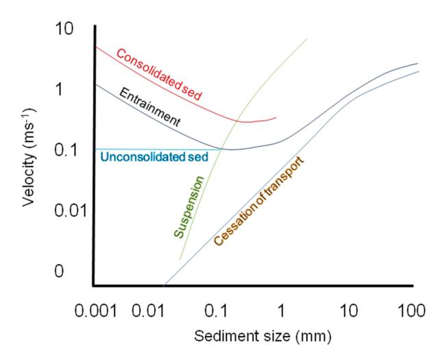
With respect to unconsolidated sediments the critical threshold for movement ( $\tau_{cr}$ ) may be calculated from the Shields entrainment function:
