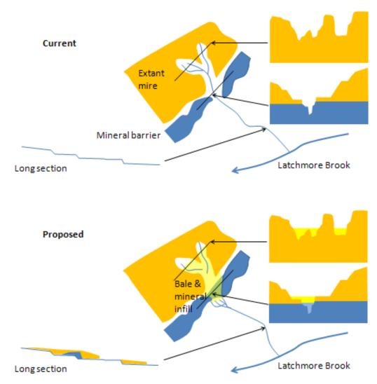
Figure 5-2: Proposed restoration for breached mineral barrier sites
