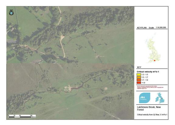
Figure 4-5b: Plot of critical velocity sites for the 2 year return period flow along the current Latchmore Brook
