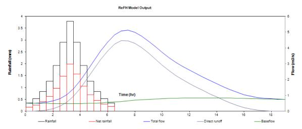
Figure 4-1: Two year flow hydrograph based on the revitalised FSR/FEH rainfall runoff method
