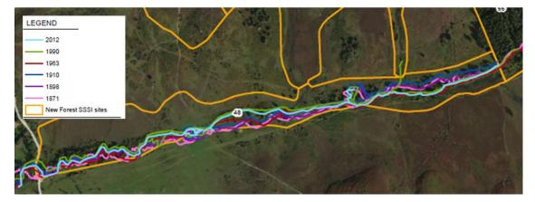
Figure 2-11: Historic channel position of Latchmore Brook based on Ordnance Survey mapping
