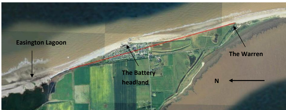
Photo 21 The Battery headland, projecting seaward from a hypothetical 2km long straight cliffline (the red line) between the Easington Lagoons and the Warren (note that the shoreline has been rotated through 90°; image source: Google Earth, image date 2008)
