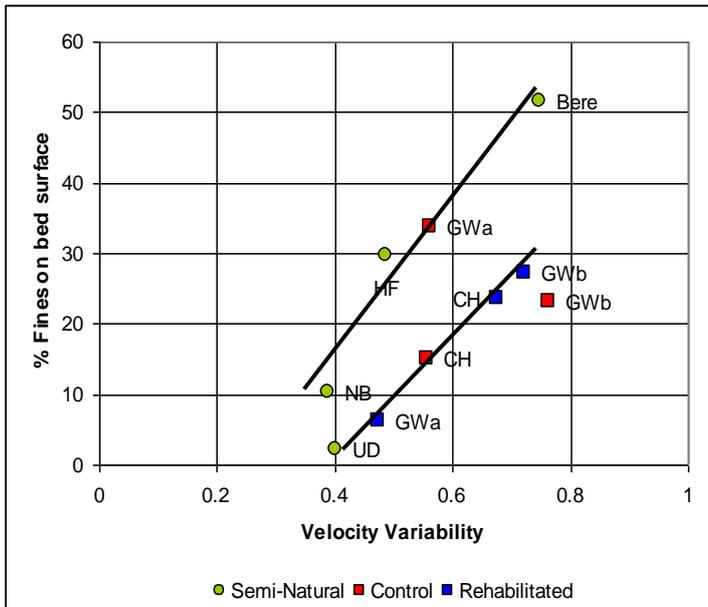
**Figure J** Relationship between the quantity of fine sediments on the surface of the river bed and the degree of hydraulic variability in a reach. The two curves, have similar slopes, but are offset due to differences in fine sediment loads in each reach . The Bere stream represents the morphologically most diverse of instream habitats (German & Sear 2003)
