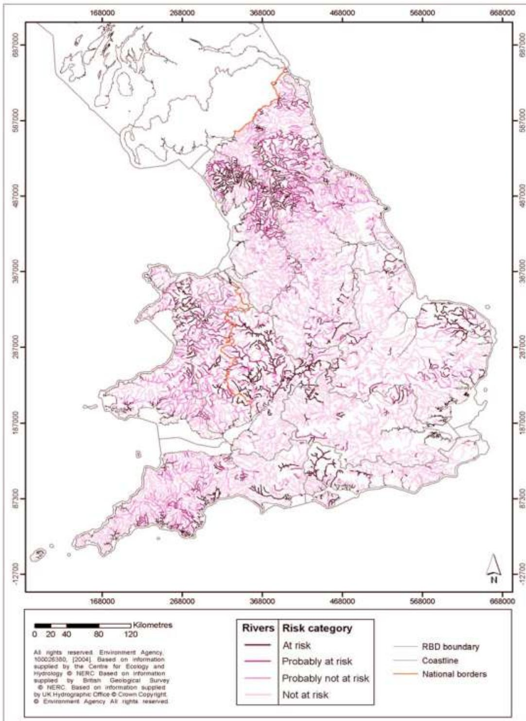
**Figure 4** River water bodies at risk of not achieving Water Framework Directive objectives due to sediment delivery pressures as identified by the Environment Agency (2004)
