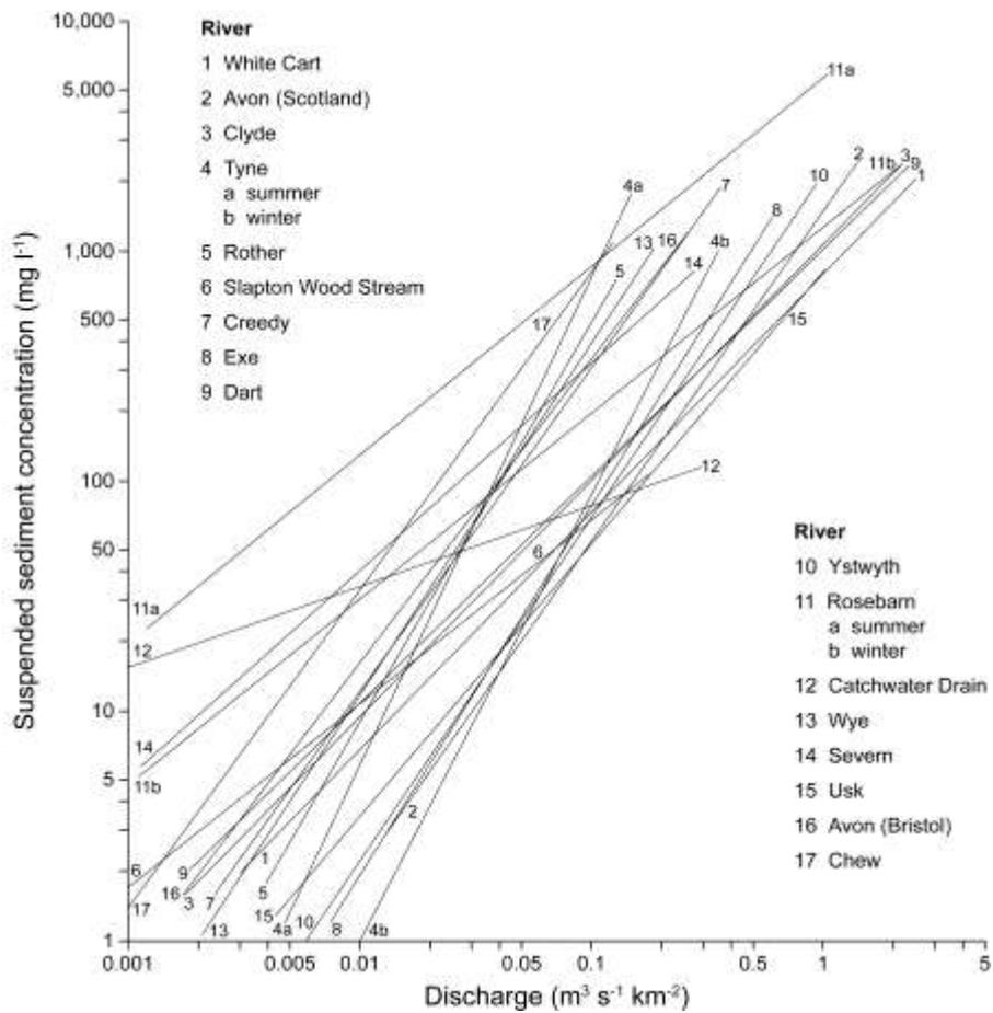
**Figure 16** A compilation of straight line suspended sediment concentration / discharge relationships or rating curves for a selection of British rivers
