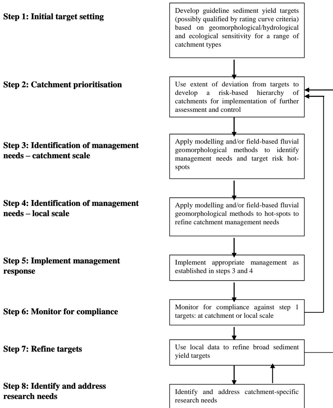
**Figure 13** Options for an operational approach to setting and applying targets: Approach 2 - a top-down approach
