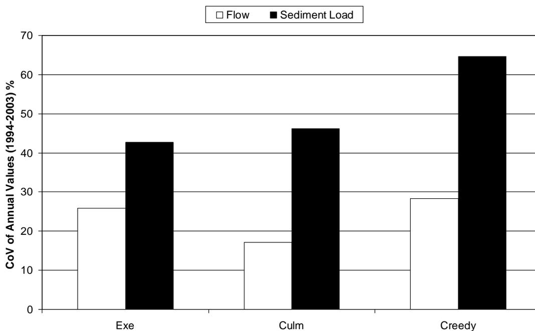
**Figure 14** The coefficient of variation of annual values of runoff and suspended sediment yield for the period 1994-2003 for the Rivers Exe, Culm and Creedy
