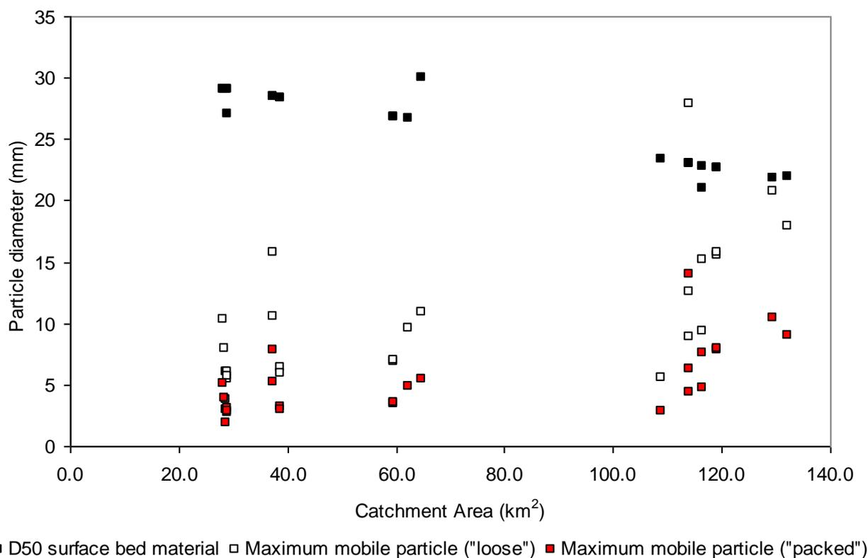
**Figure C** Gravel bed stability in the River Nar, Norfolk based on estimated maximum particle mobility using Shields entrainment function
