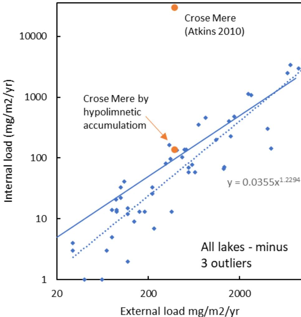
**Figure 12. A simple empirical model based on the data of Nurnberg 1984 using only sites with positive internal loads. Note the log-log scale. Dashed line is the line of best fit (power), and the solid line represents  $L_{\text{internal}} = 0.25 \times L_{\text{external}}$**
