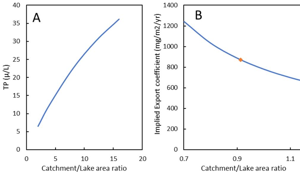
**Figure 5. The impact of catchment to lake area ratio on: A) lake water TP. B) Estimated diffuse P loads (expressed as an export coefficient) calculated from measured TP. The orange diamond represents our best estimate of the catchment to lake area ratio at White Mere**
