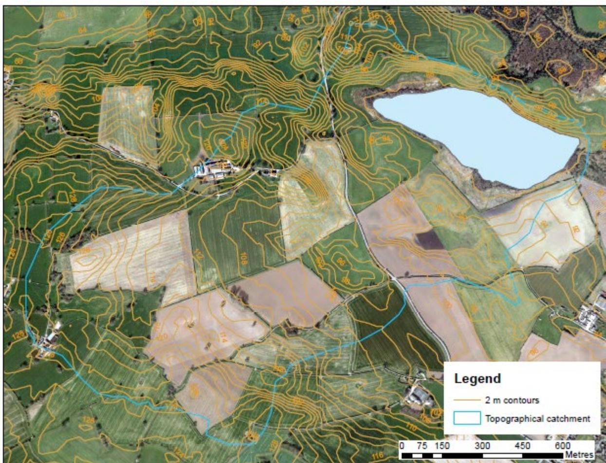
Figure 1. Topographical map of Crose Mere, with 2 m LIDAR-based contours superimposed on the 2012 Air photograph
