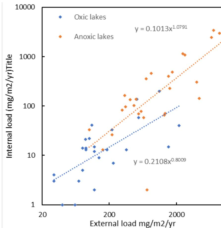
**Figure 11. The dependence of internal P load on external P load. Data from Nurnberg (1984). To create this log-log plot all sites with 0 or negative apparent internal P load are excluded. Thus, the plot represents sites with relatively high internal loads, and may be regarded as an upper limiting rate**
