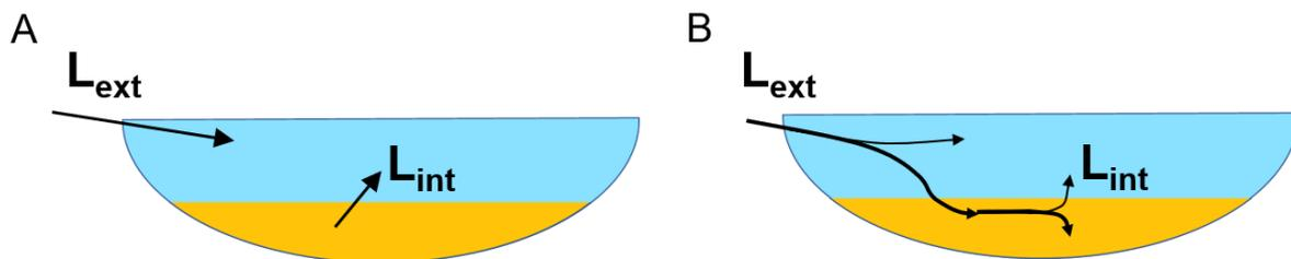
**Figure 10. External ( $L_{ext}$ ) and internal ( $L_{int}$ ) loading viewed over two timescales. A, The short term view (~annual) considers  $L_{ext}$  and  $L_{int}$  as two separate sources; B, the long term (~decadal) view considers  $L_{ext}$  and  $L_{int}$  as linked sources where  $L_{int} = f(\text{historical } L_{ext})$  and  $L_{int} < \text{max. historical } L_{ext}$ .**
