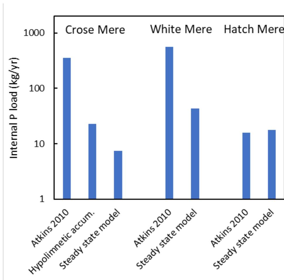
**Figure 13. A comparison of internal P load estimates for the three lakes. Steady state model refers to the empirical model from Figure 12. Note log scale**
