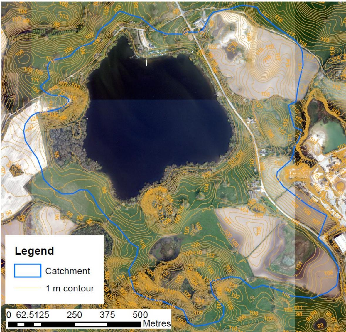
**Figure 17. Topographical map of White Mere, with 1 m LIDAR-based contours superimposed on the 2012 Air photograph**
