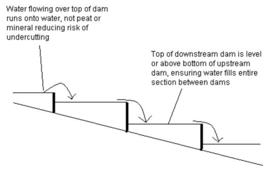
Figure 3-33: Spacing of Dams in a Gulley (from Evans et al., 2005)
