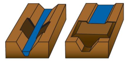
Figure 3-3031: Installation of a peat plug (from Quinty and Rochefort, 2003)
