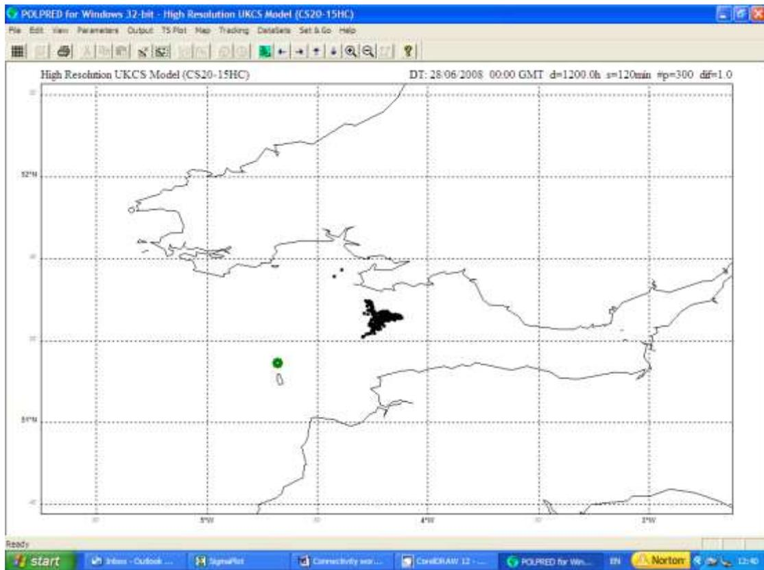
**Figure 6:** Typical model output for a run using POLPRED 2.0 tidal prediction software. The circle shows the point of release for 300 particles (= eggs) which were tracked dispersing on tidal currents for a period of 50 days. Squares show the points reached by each particle by the end of this dispersal period.
