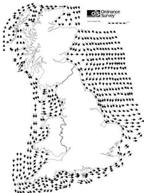
**Figure 4:** Current Vector Map for Great Britain showing typical average annual directions of residual currents. The length of the arrows is proportional to current speed. Data from IACMST (2005) and DTI (2004).
