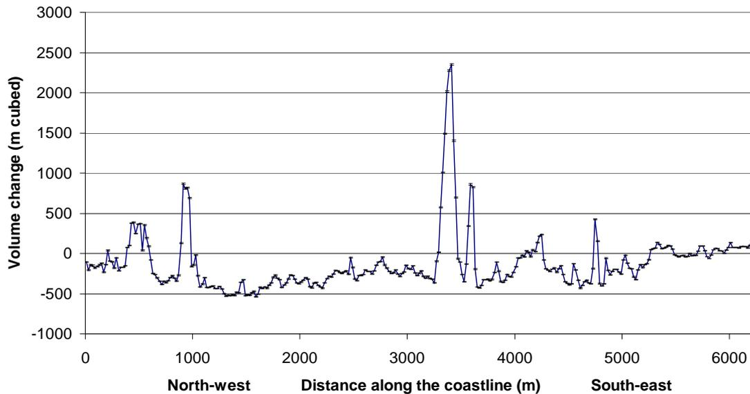
**Figure 10 Shingle ridge volume change (2006-2008), calculated at 20 m intervals along the coastline. Error bars are 95% confidence intervals**
