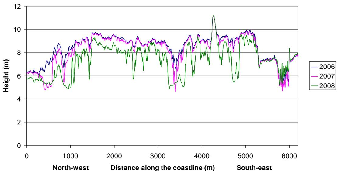
**Figure 5 Changes in the maximum height of the shingle ridge between 2006 and 2008 (calculated at 2 m intervals along the coastline)**
