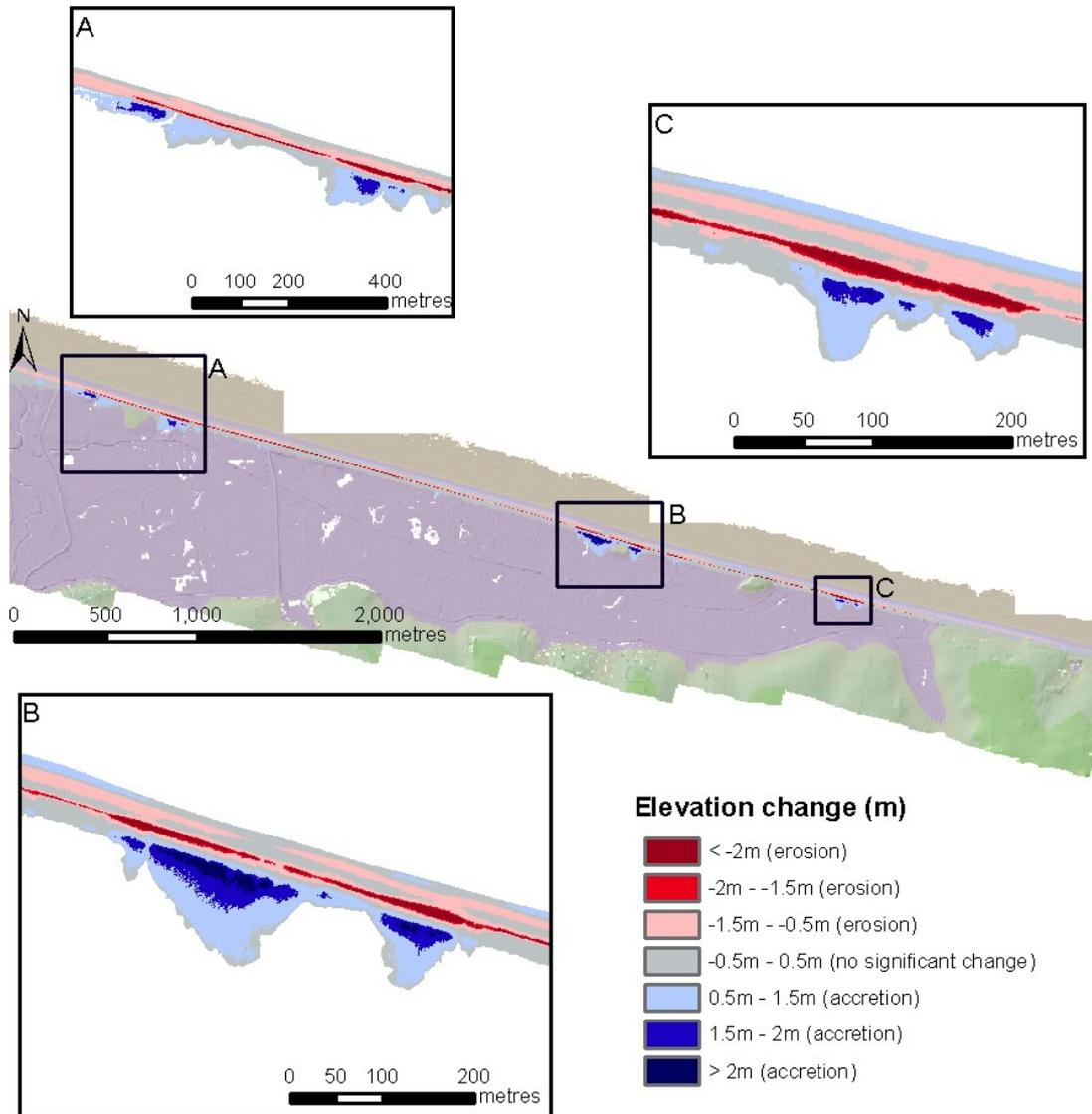
**Figure 9 Elevation change of the Cley shingle ridge (2006-2008). The imagery is the LIDAR from 2007**
