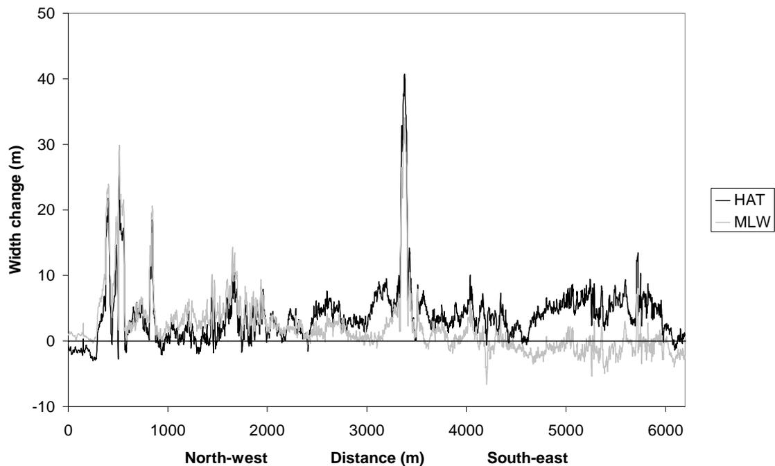
**Figure 13 Width change between 2006 and 2007, using HAT (black line) and MLW (grey line) to define the seaward extent of the ridge**
