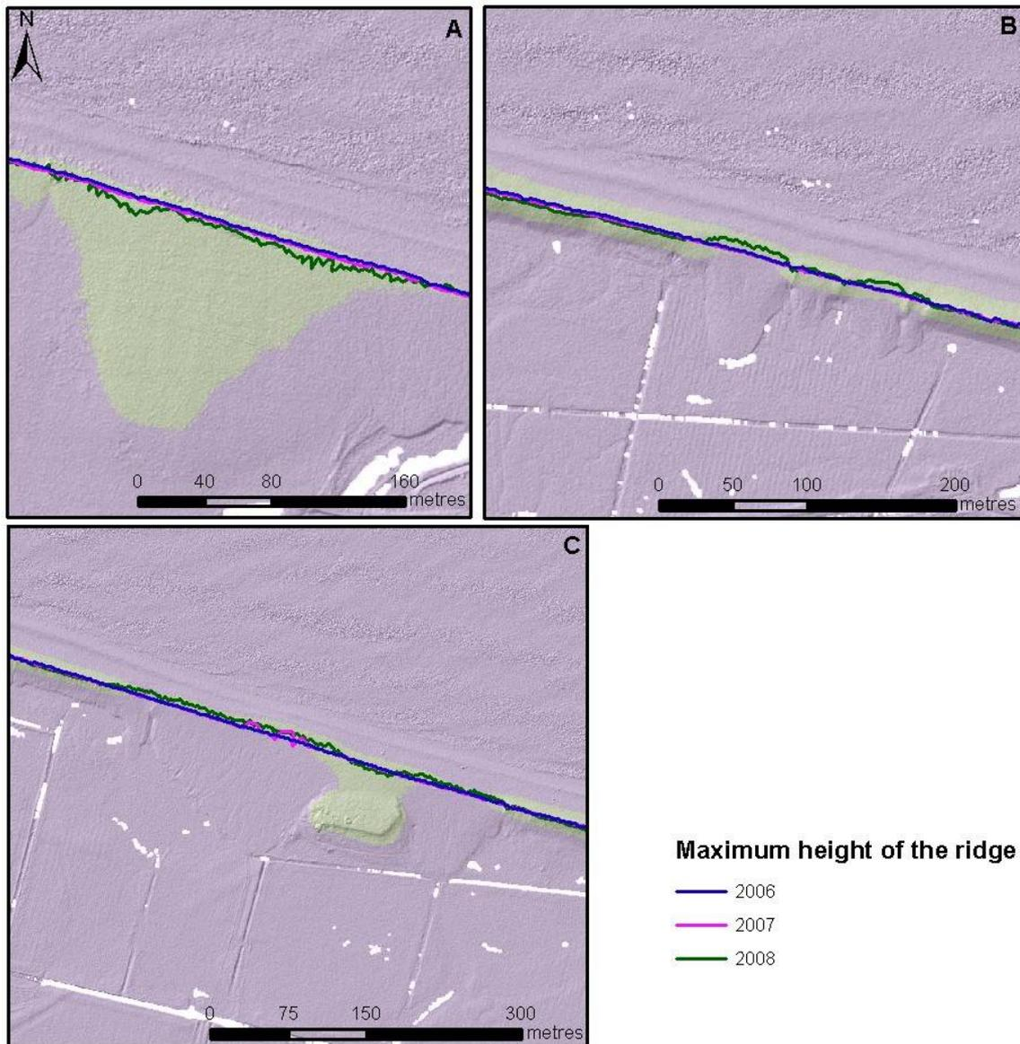
**Figure 6 Location of the maximum height of the ridge between 2006 and 2008 for three small sections of the ridge. The imagery is the LIDAR data for 2008**
