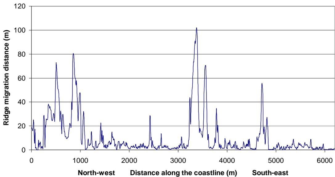
**Figure 8 Migration of the landward extent of the shingle ridge between 2006 and 2008 (calculated at each 2 m interval)**
