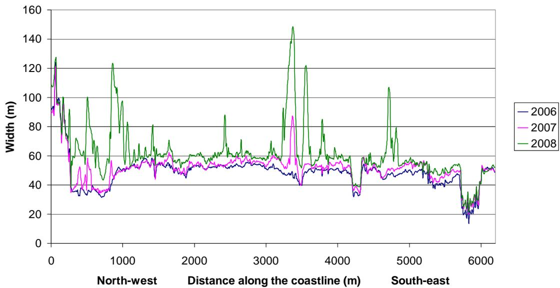
**Figure 7 Changes in the width of the shingle ridge between 2006 and 2008 (calculated at 2 m intervals along the coastline)**
