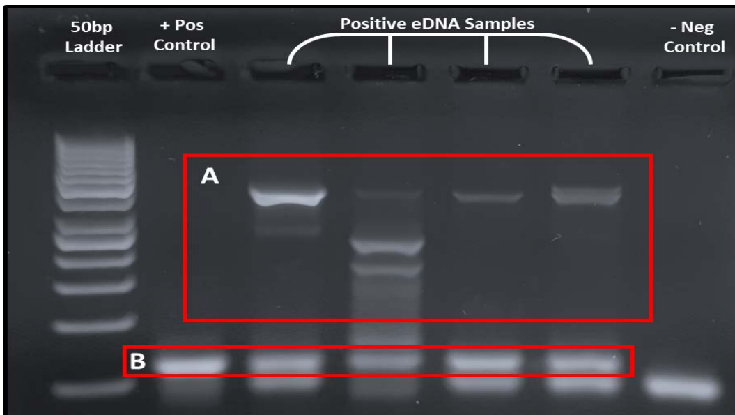
Figure 9. Gel image of qPCR product from crayfish plague eDNA detection demonstrating non-specific amplification indicated by additional bands of amplified DNA (A) in the region of 150-400bp to the expected bands (B) at 59bp.
