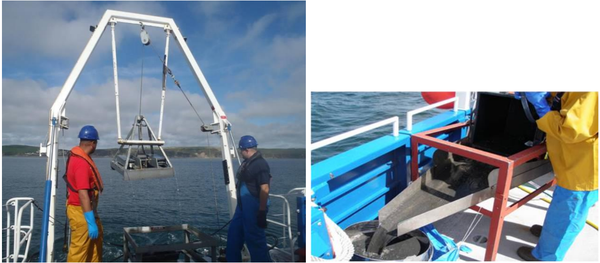
Figure 7. Mini-Hamon Grab (left), and equipment for sieving benthic fauna samples (right).
