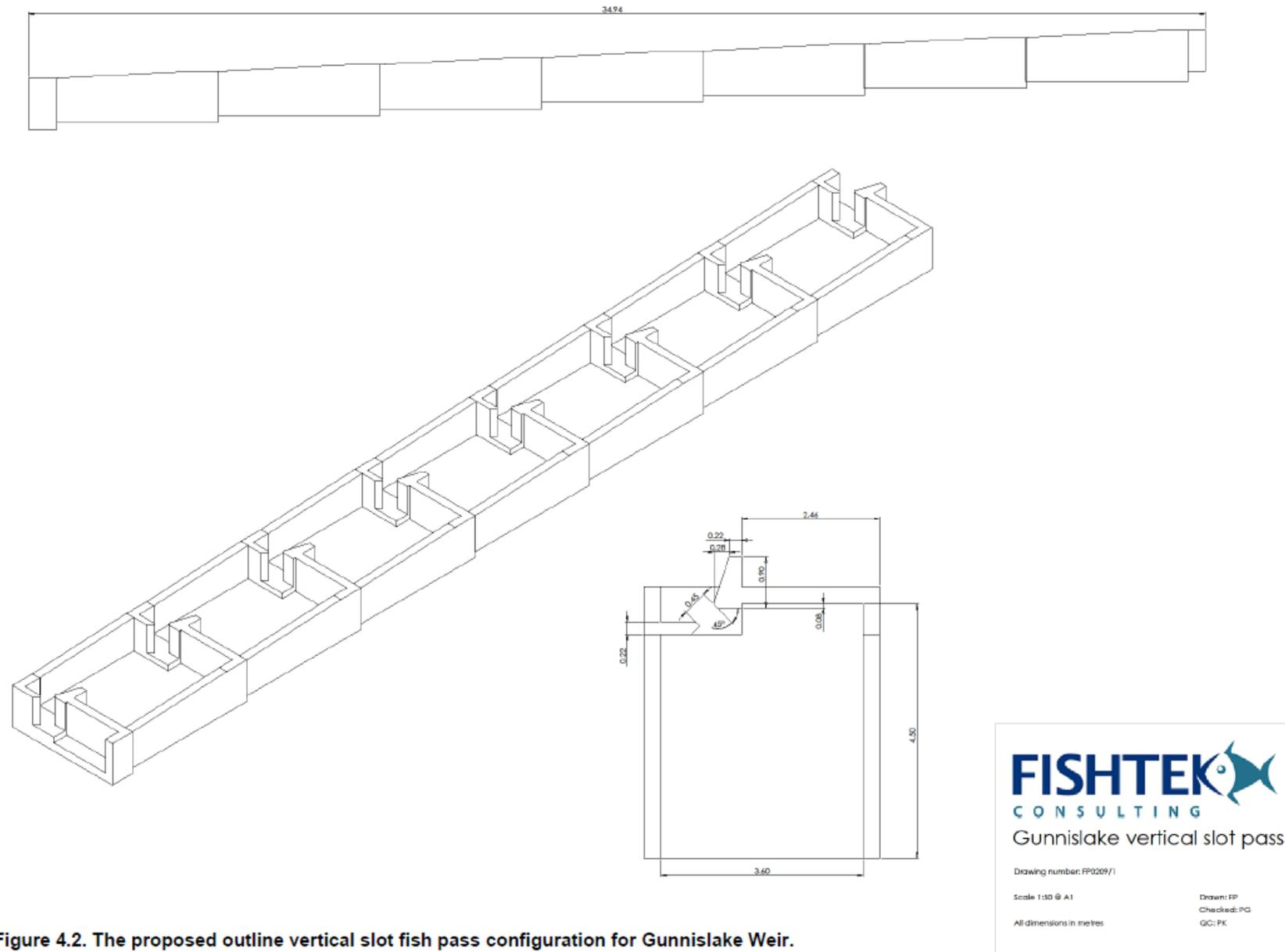
Figure 4.2. The proposed outline vertical slot fish pass configuration for Gunnislake Weir.
