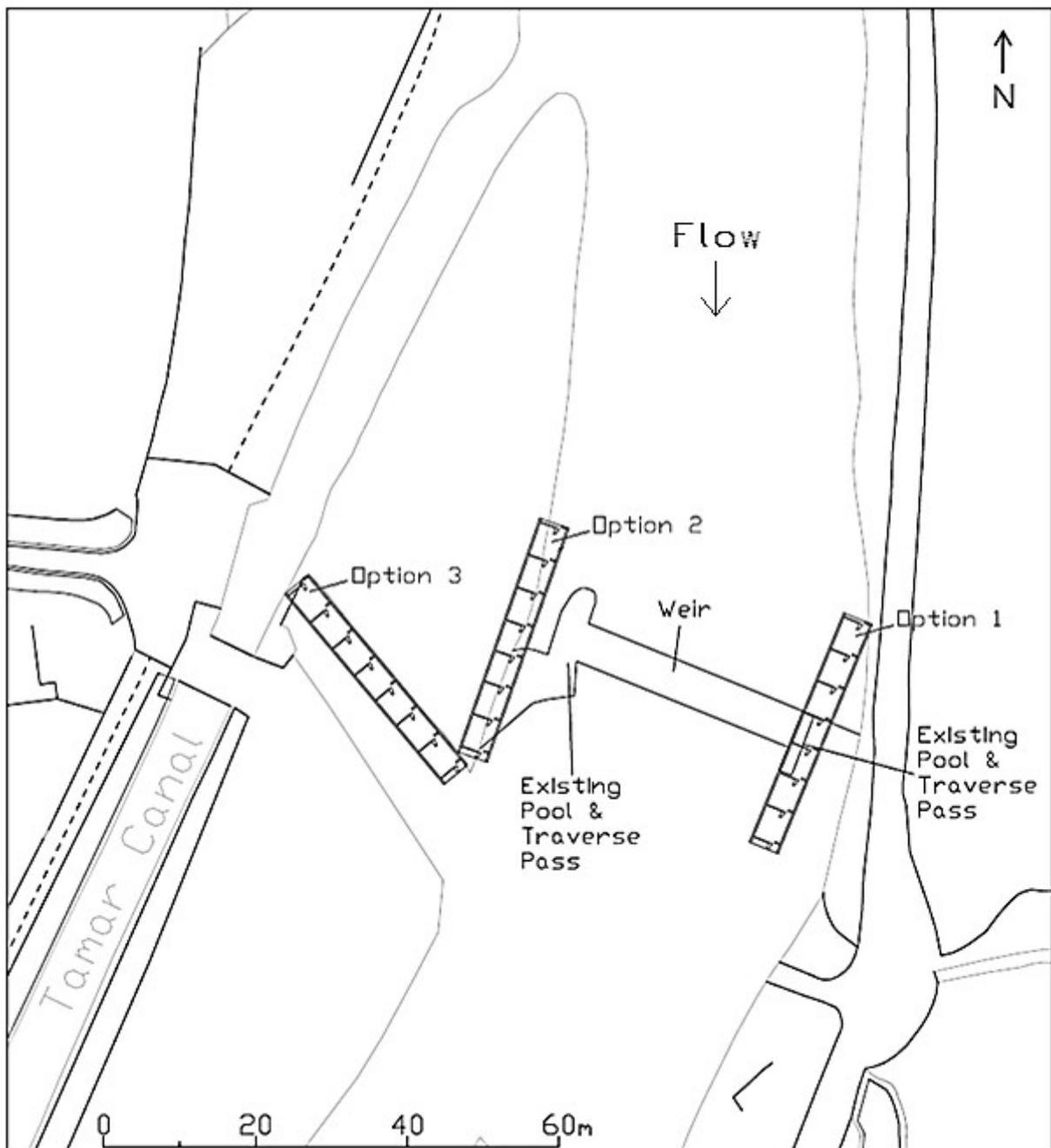
**Figure 4.1. The three possible locations considered for the vertical slot fish pass on Gunnislake Weir during the second site visit.**
