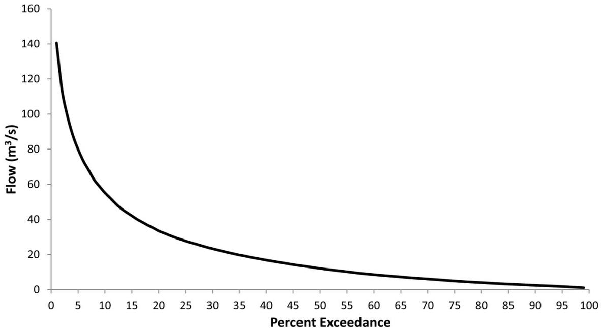
**Figure 1.2. A flow duration curve for the River Tamar at Gunnislake gauging station (station number 47001) based upon long-term gauging data (1956 – 1990).**
