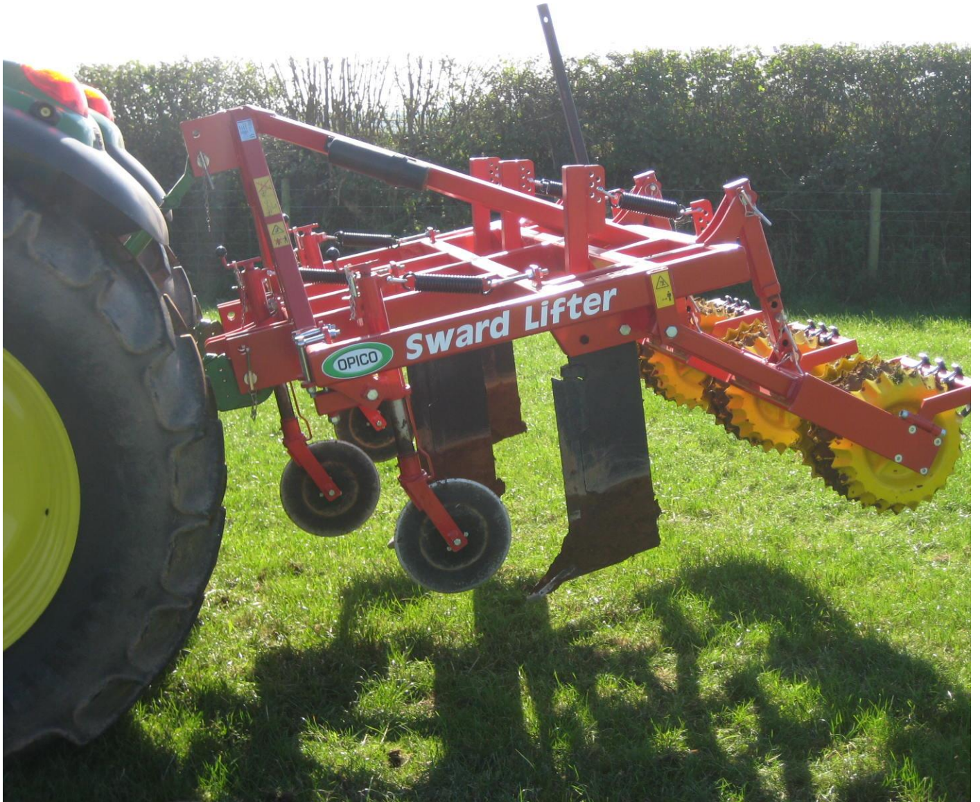
A Sward Lifter being demonstrated to a group of farmers during a Soils for Profit Project farmer training event on Bodmin Moor
