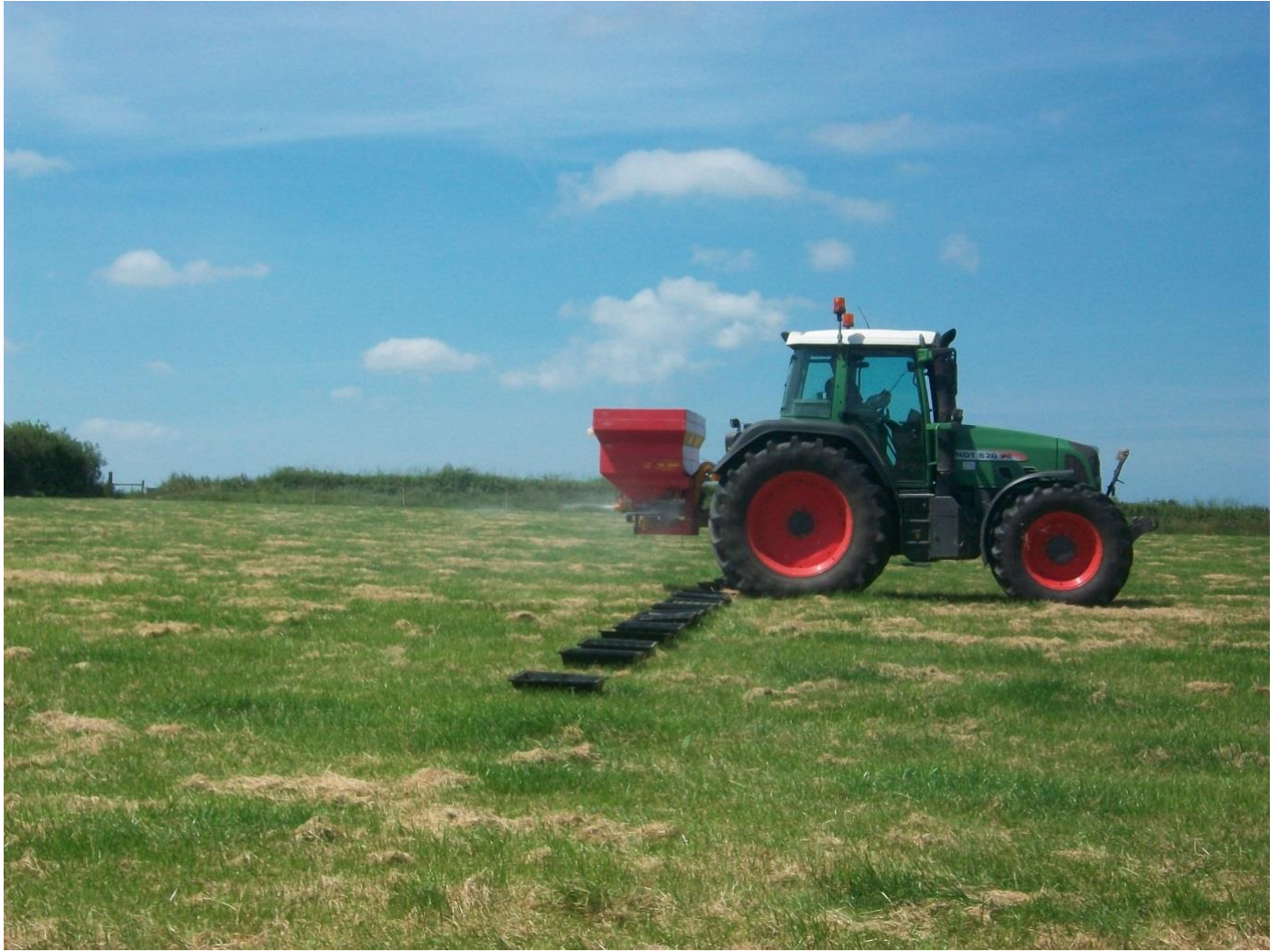
Demonstration of a tractor & fertiliser applicator being driven between trays so that the applicator can be assessed for evenness of fertiliser spread and then calibrated if necessary.
