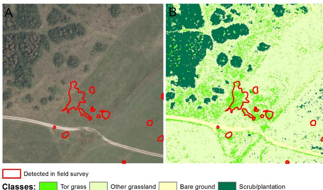
**Figure 5.** Example surveyed 200 m x 200 m square, showing **A)** summer 2014 aerial photography and **B)** maximum likelihood classification. Both images are overlain with current (January 2015) *Brachypodium* agg. cover as detected in field survey (red outlines). Whilst bare ground and scrub are well separated, *Brachypodium* agg. is frequently misclassified, with both false positives and false negatives.
