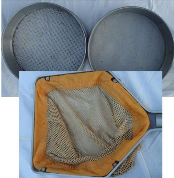
Figure 9. 10mm / 2mm grade 30cm sieve nest and 2.5mm mesh net for sampling for C. chinensis (© Dr Martin Willing)
