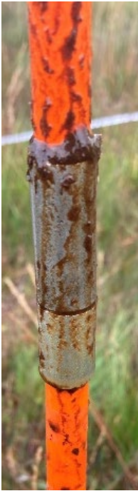
Photo 2. Soil collected on the join between two probe sections. © Natural England
