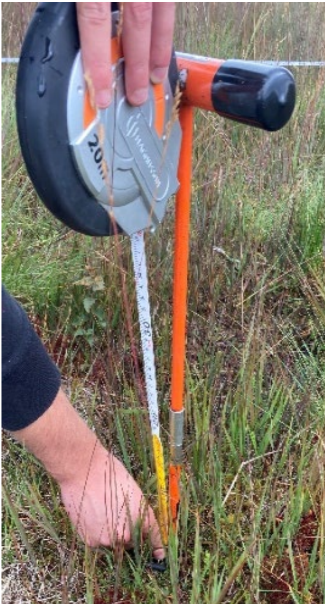
Photo 1. Measuring from the ground upwards to the end of the probe. © Natural England
