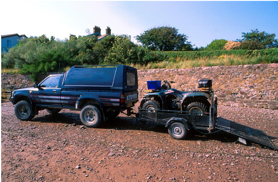
Yamaha Kodiak ATV equipped with differential GPS
