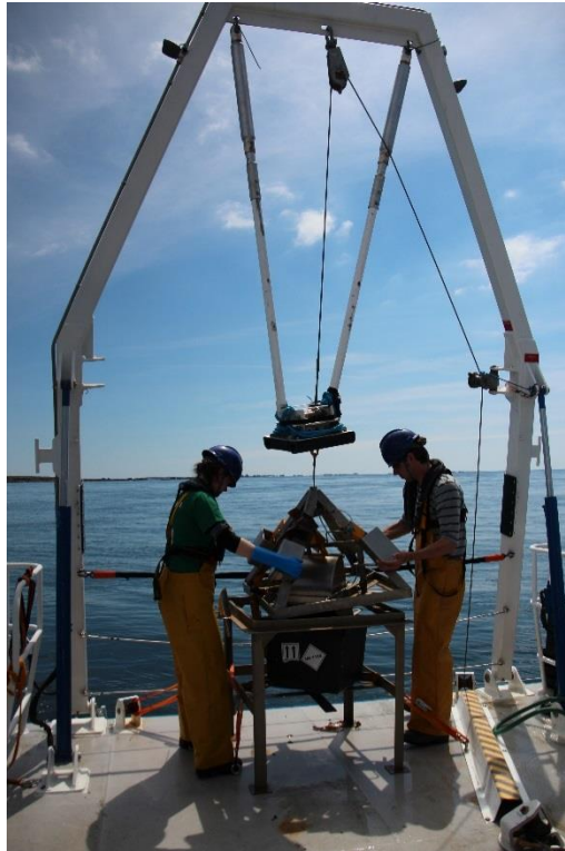
Figure 4. Day Grab being deployed from the stern of the vessel.
