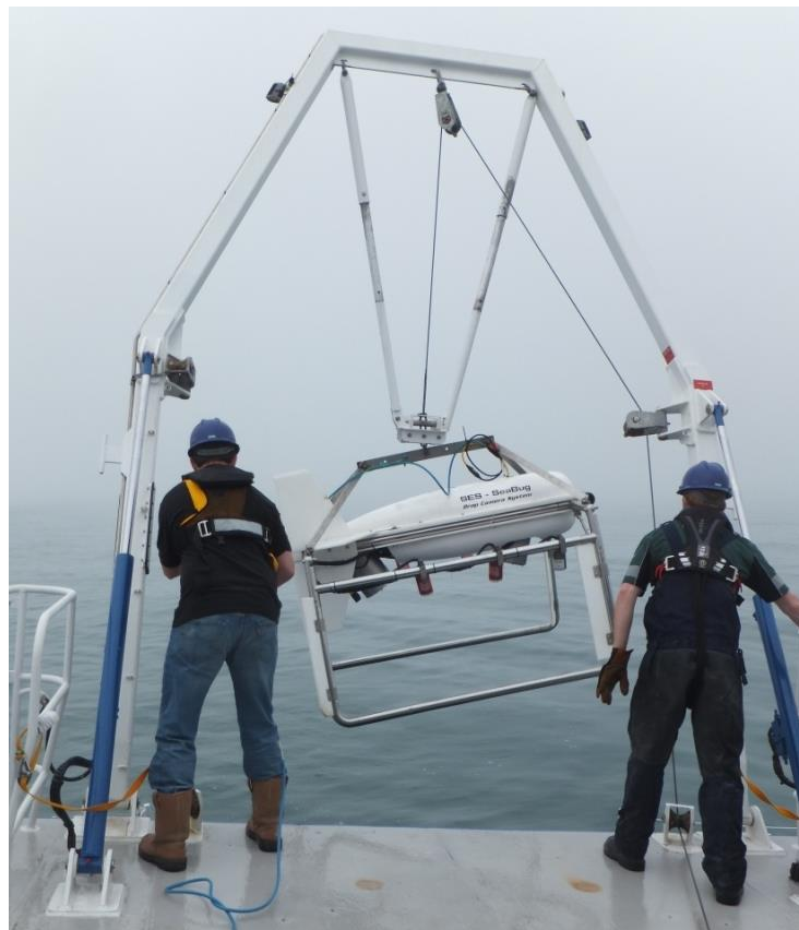
Figure 6. Seabug drop camera system being deployed from the stern of the coastal survey vessel.
