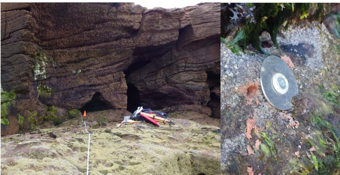
Figure 32: a) Top of transect in small cave and b) New marker bolt on the side of the cave at Brotherston's Hole in the Berwickshire and North Northumberland Coast Special Area of Conservation
