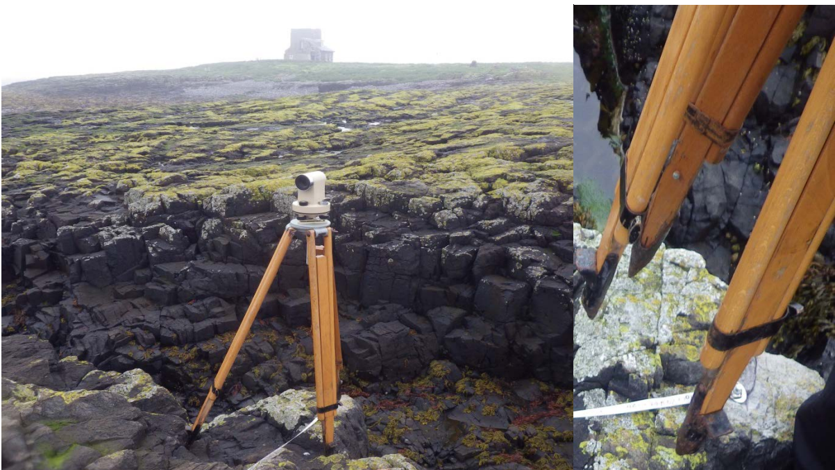
Figure 20: a) Location placer shot in front of the warden's cottage and b) New marker bolt on the top of the bedrock on Brownsman in the Berwickshire and North Northumberland Coast Special Area of Conservation
