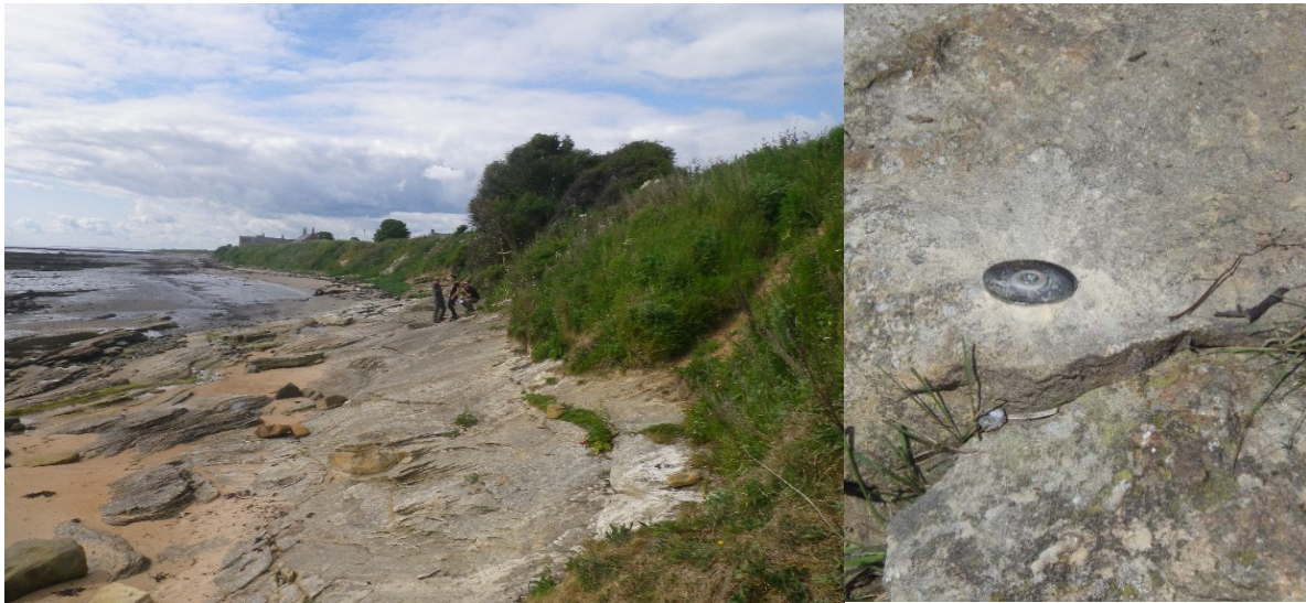
Figure 4: a) Access onto the shore down the low vegetated cliffs and b) New marker bolt on the top of the bedrock alongside the old screw marker at Boulmer in the Berwickshire and North Northumberland Coast Special Area of Conservation
