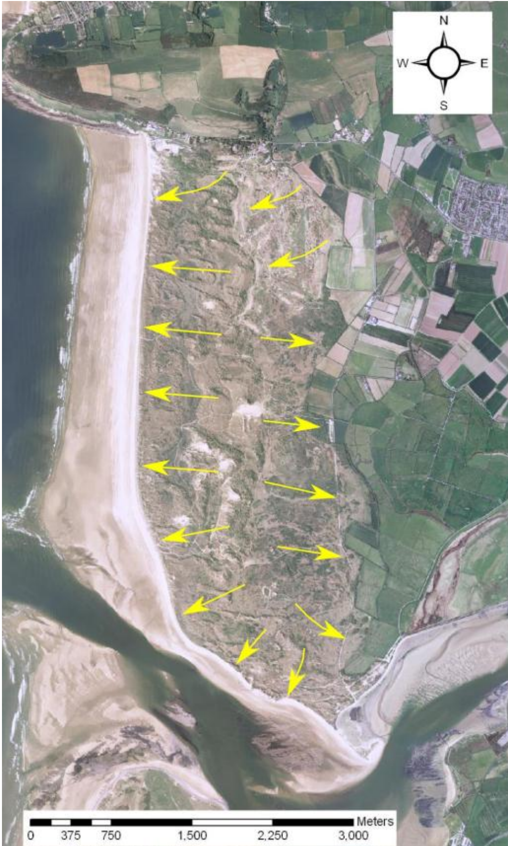
Figure 6. Braunton Burrows conceptual groundwater flow diagram. The yellow arrows indicate the direction of groundwater flow. © NERC (CEH) 2013, © NextPerspectives.
