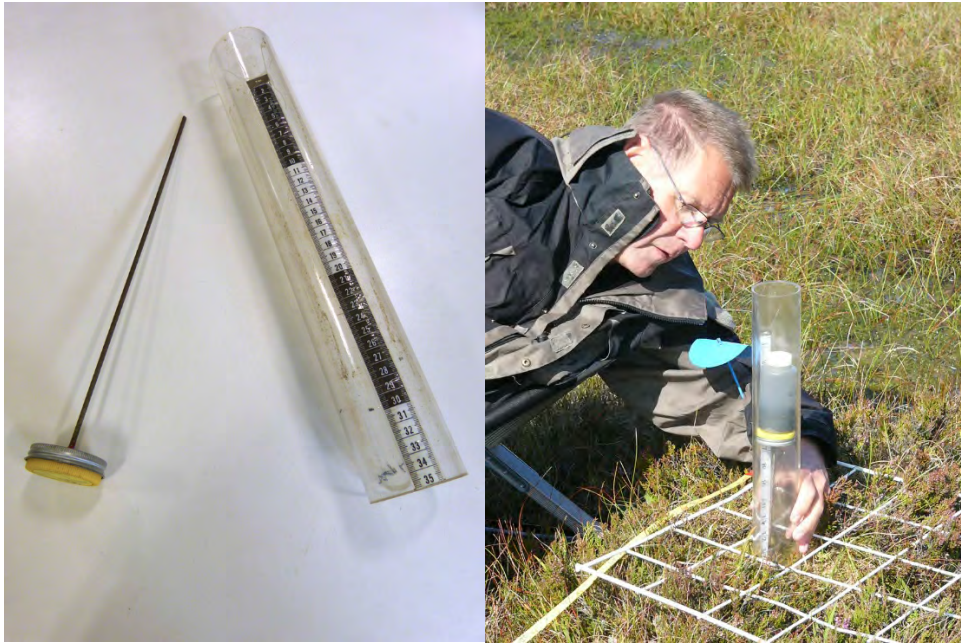
Figure 27 Penetrometer for use on peat soils. (left) Components of the penetrometer. (right) Penetrometer in use in the field.
