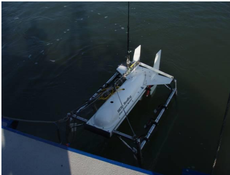
Figure 4. STR SeaBug drop Camera being deployed from the stern of the coastal survey vessel.
