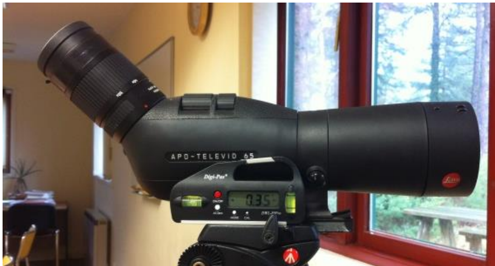
Figure 1: Telescope and inclinometer
