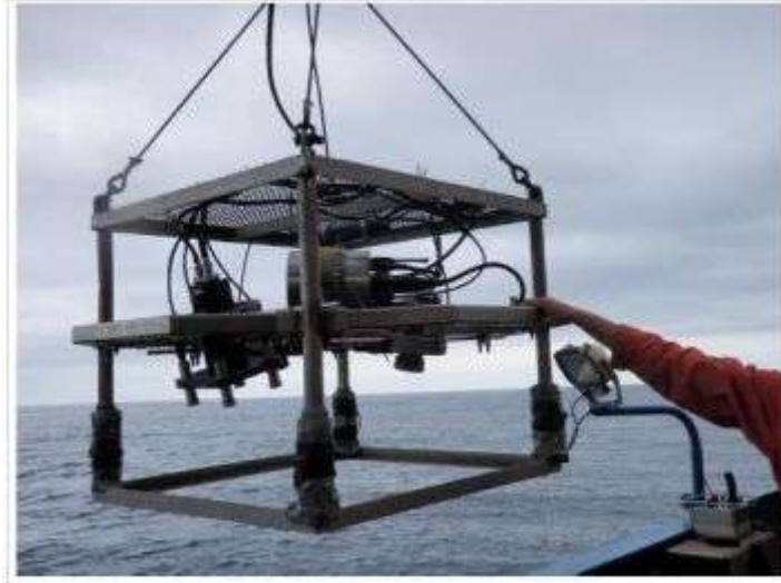
Figure 3 Drop camera frame with video and stills cameras and lighting configured according to MESH ROG
