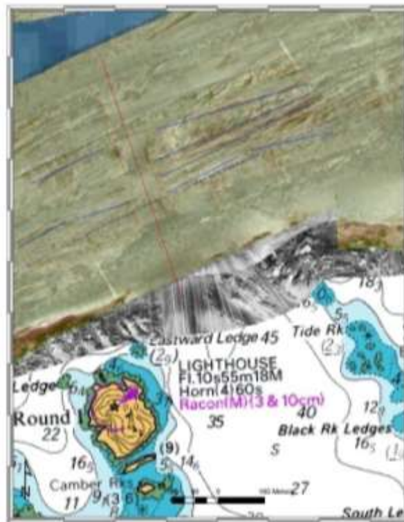
Figure 7. Sediment filled channel feature (red line) cutting through ledges (Blue lines) off Tean Sound
