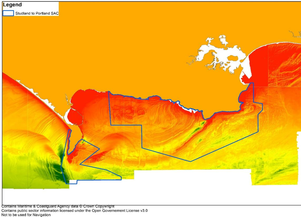
**Figure 2. Bathymetry collected and compiled as part of the Dorset Integrated Seabed Study overlaid with the Studland to Portland SAC.**
