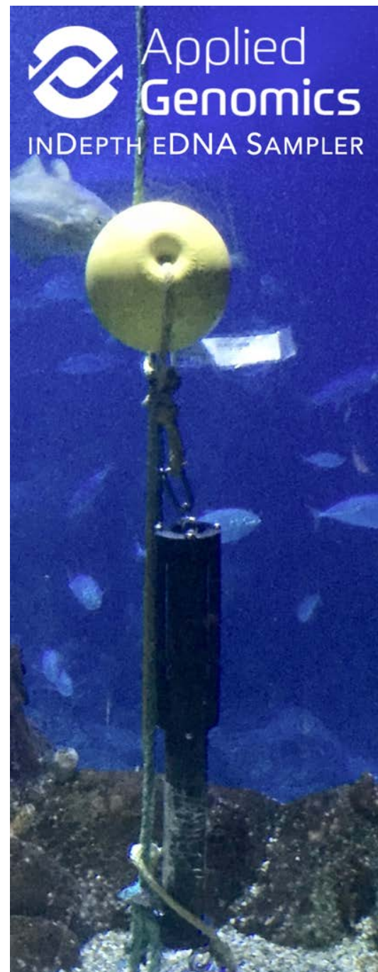
Figure 1: The Applied Genomics inDepth eDNA Sampler is capable of filtering 50 litres of seawater at greater than 150 metres depth over several tidal cycles.
