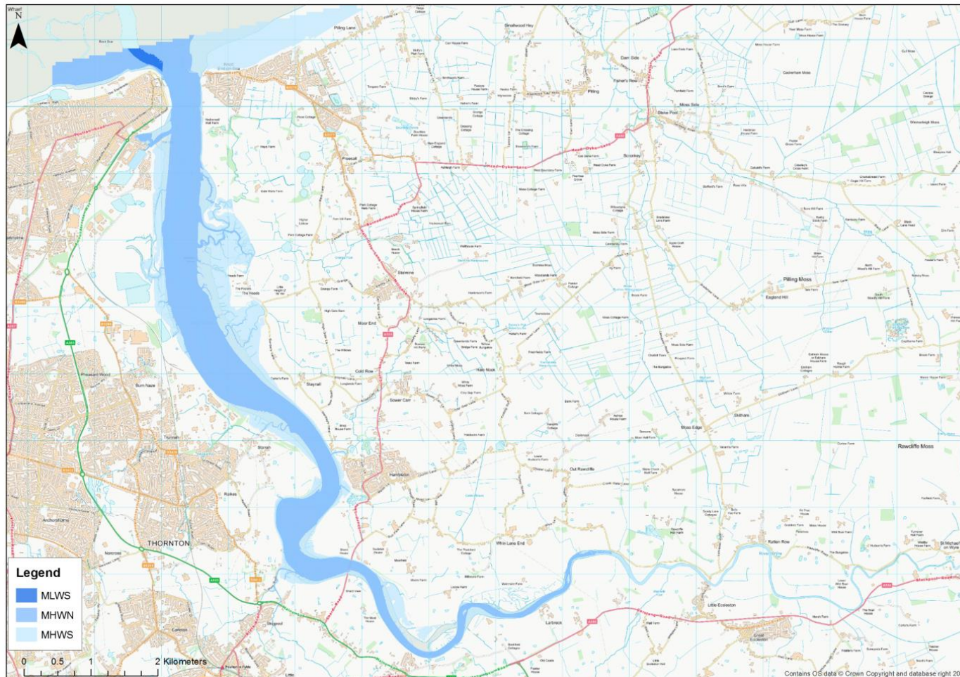
Figure 0.19. Tidal datums in the Wyre Estuary. Note that there is no slicing at MLWS because its elevation could not be extracted from the LiDAR data
