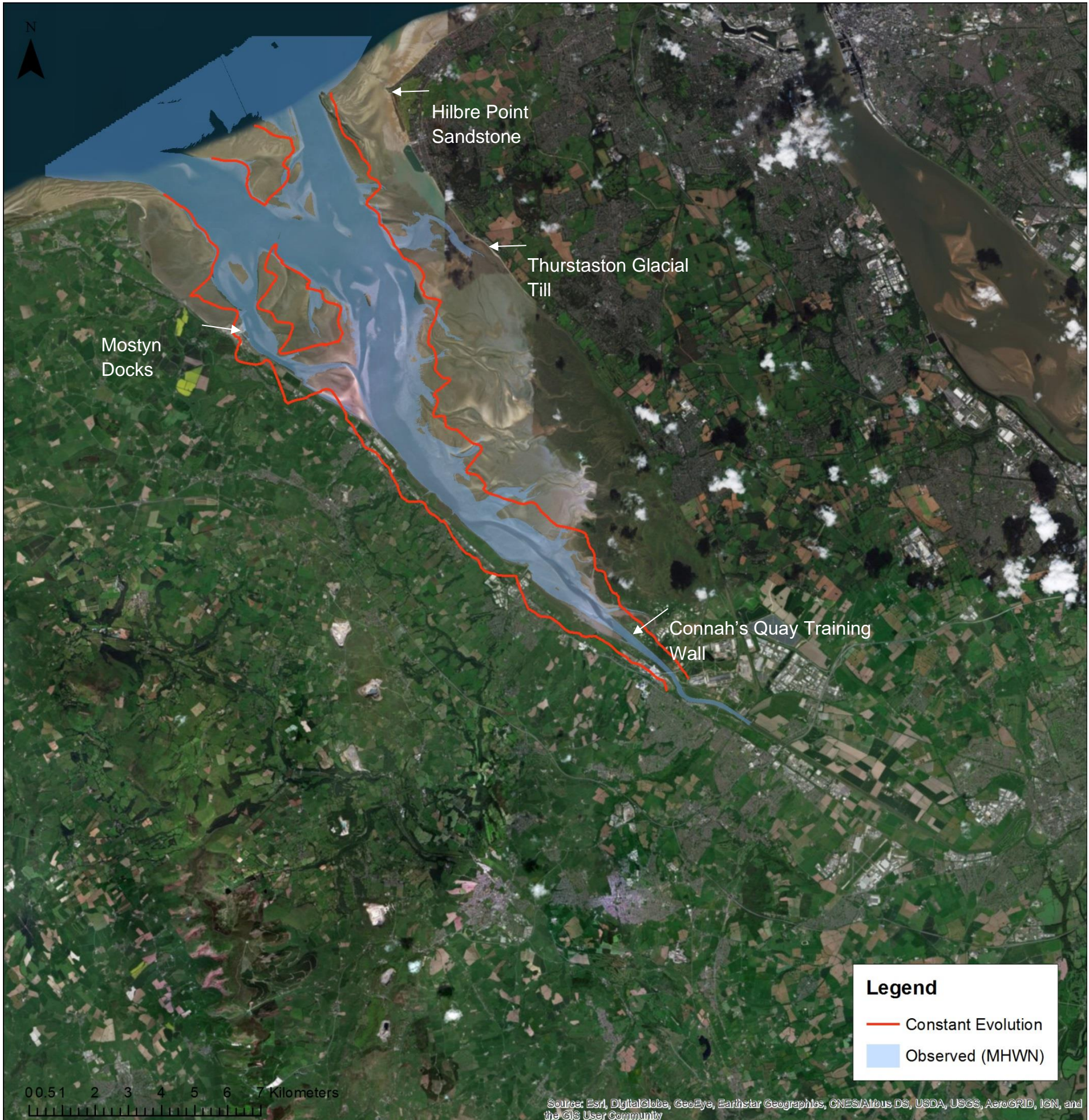
Figure 0.9. Comparison of predicted equilibrium widths with observed widths in the Dee Estuary (aerial photograph background)
