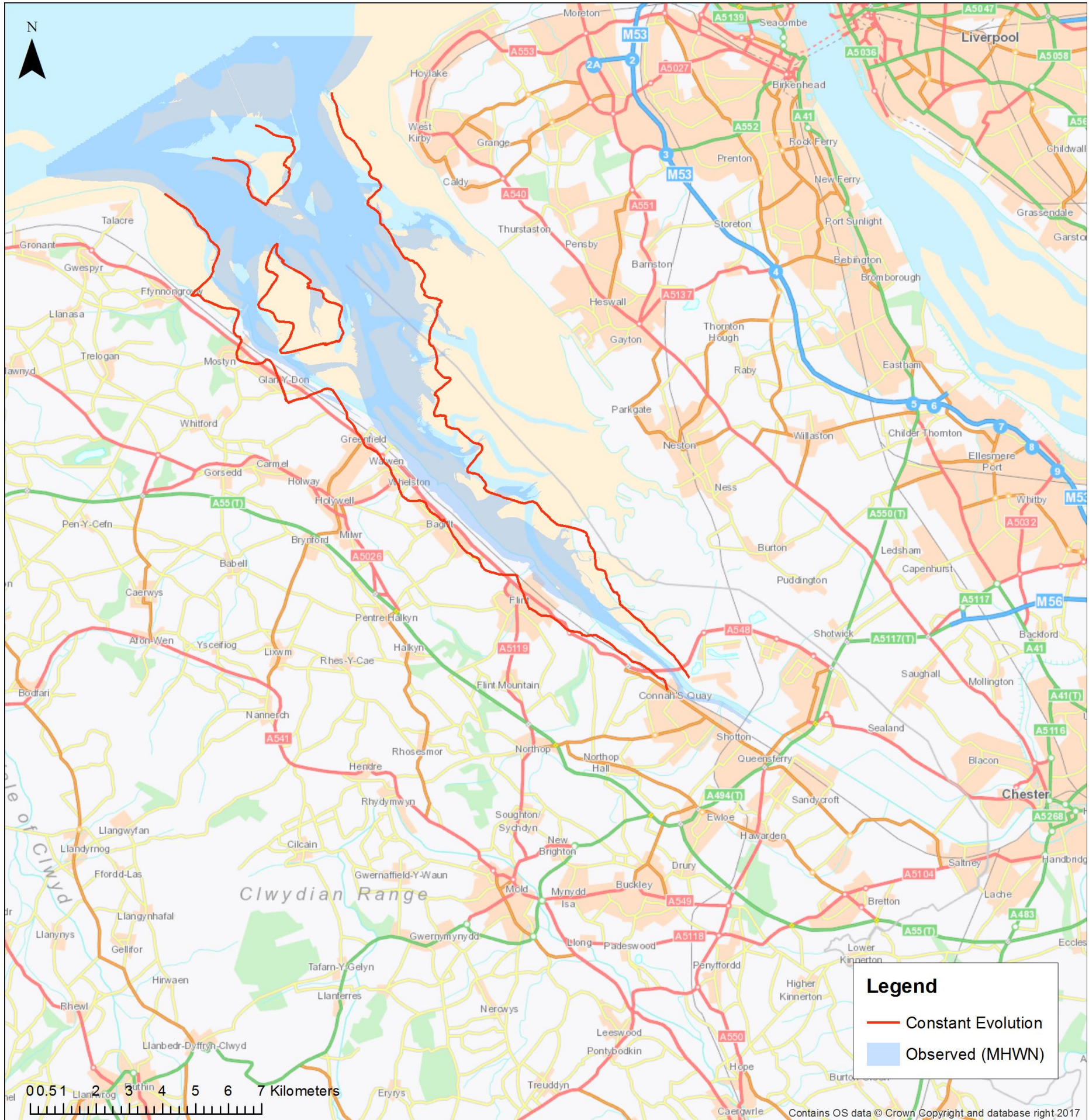
Figure 0.8. Comparison of predicted equilibrium widths with observed widths in the Dee Estuary (map background)
