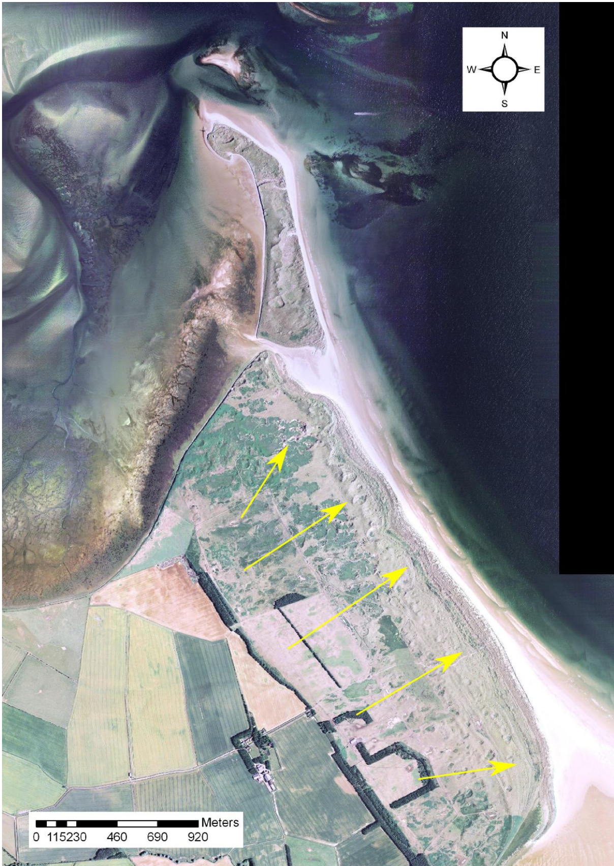
Figure 5. Ross Links conceptual groundwater flow diagram. The yellow arrows indicate the likely direction of groundwater flow. © NERC (CEH) 2013, © Next Perspectives.
