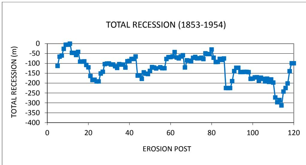
**Figure 49 Holderness cliffs: total cliff recession at Erosion Post (EP) locations, 1853-1954 (data for the EPs are from the nearest beach profile site, generally within 100-200m)**
