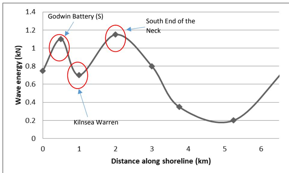
**Figure 5** Longshore wave energy gradient along Spurn seaward shoreline (adapted from IECS, 1992). A positive longshore power gradient (i.e. increasing wave energy) indicates shoreline erosion, whereas a negative gradient (i.e. decreasing wave energy) indicates deposition.
