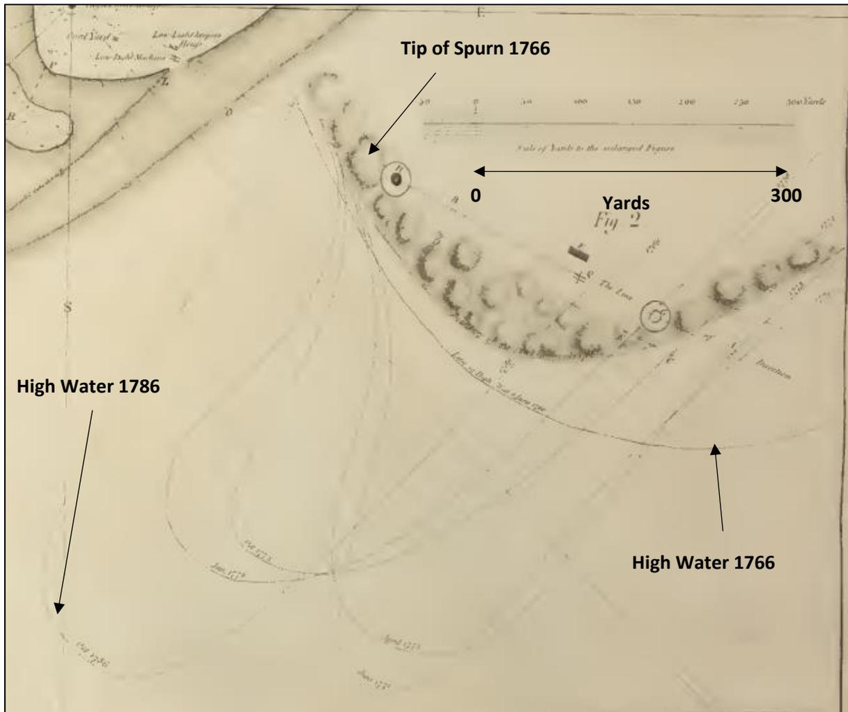
**Figure 8 Changes in the tip of Spurn between 1766 and 1786 (from Smeaton 1791, with additional labels)**
