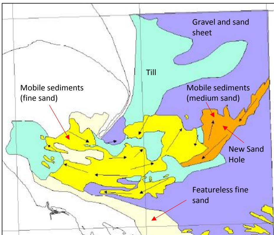
Figure 32 Seabed sediments map of the Humber mouth, black arrows indicate sediment transport directions (after Balson and Philpott 2004)
