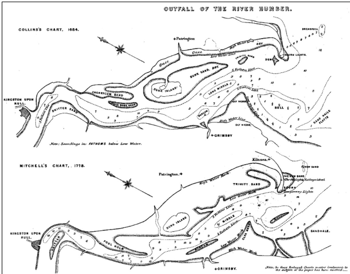
Figure 11 The impact of land reclamation at Sunk Island on the North Channel, between 1684 (top) and 1778 (bottom chart).
