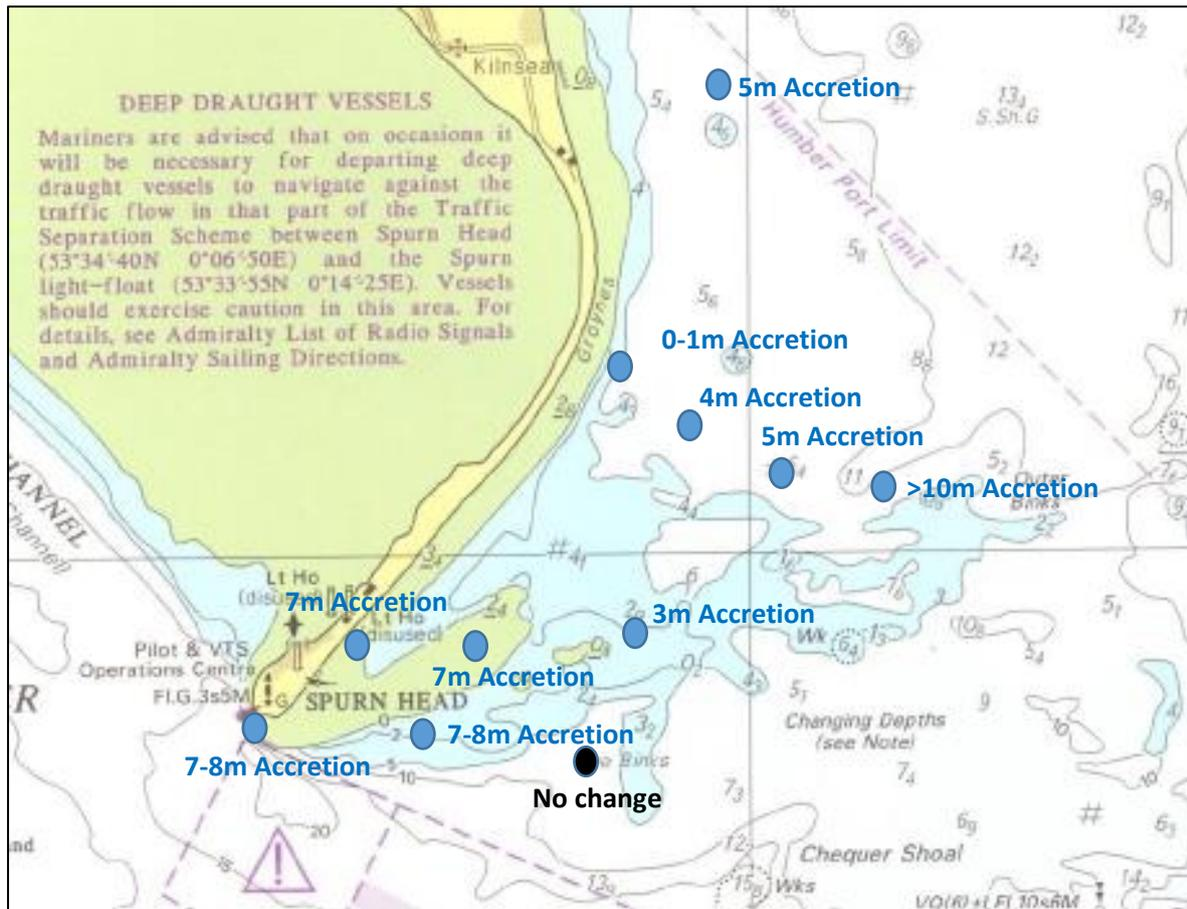
Figure 41 Comparison of the present day water depths with depths records by Greenville Collins on his chart of 1684. Blue dots are the approximate locations of Collin’s soundings; the labels indicate the amount of accretion since the 1680’s. (note that the Chart Datum is not stated and are assumed here to be to -2.7mOD, rather than the modern chart datum of -3.9m)
