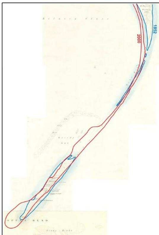
**Figure 42 Comparison of the 1852 (blue line; this shows the spit following the 1849/50 breach) and 2000 (red line) shoreline positions along Spurn (from Pye and Blott, undated)**
