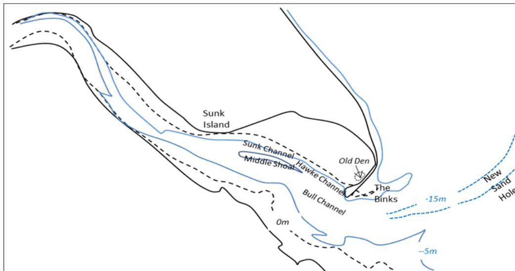
Figure 47 The Outer Humber and its approaches, showing features mentioned in the text. Isobaths depths refer to Admiralty Chart Datum at -3.9mOD
