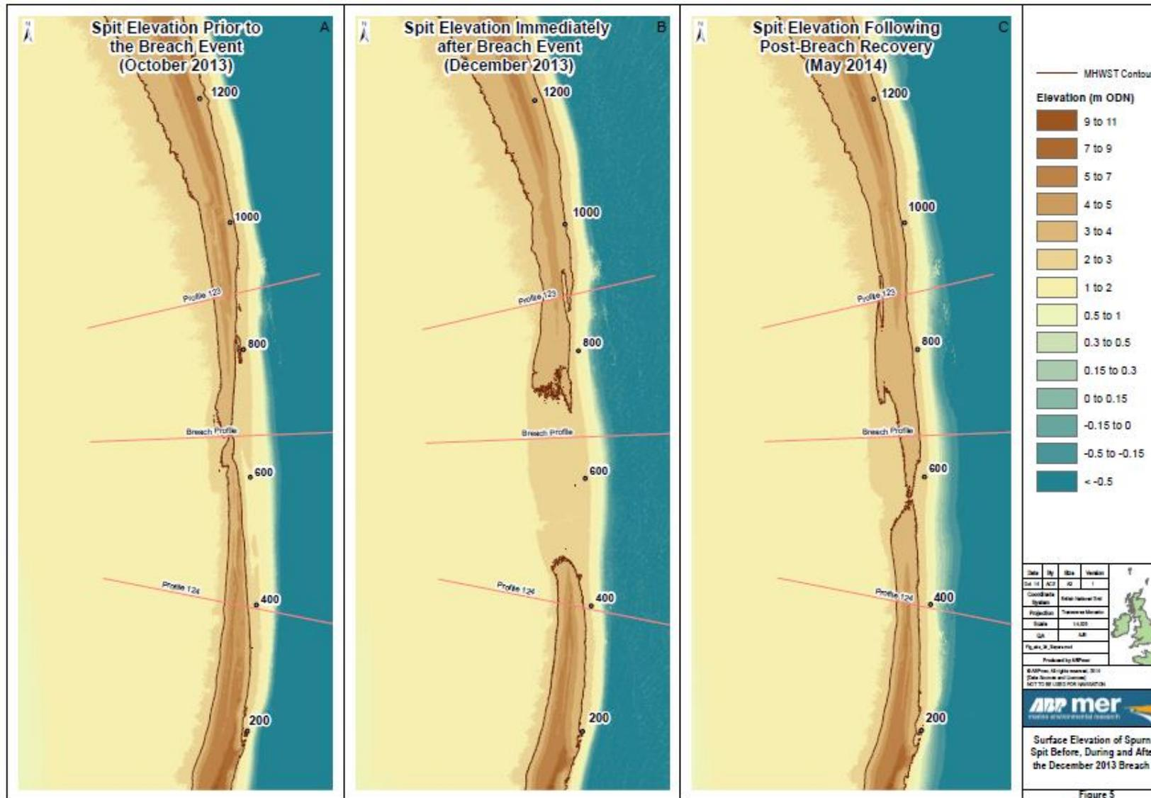
Figure 24 Surface elevation of Spurn prior to and after the 2013 temporary breach (from ABP mer 2014)
