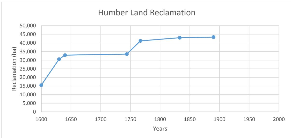
Figure 12 The post 1600 cumulative history of land reclamation in the Humber (the value at 1600 is for the Hull valley, believed to have been reclaimed earlier in the Millennium).
