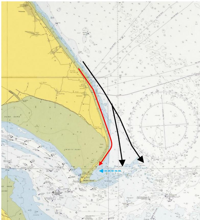
**Figure 3 Coarse sediment transport pathways around Spurn: black lines indicate the transport pathway in 5-10m water depth; red line indicates the longshore transport on the beach; blue line is a conjectured onshore route.**
