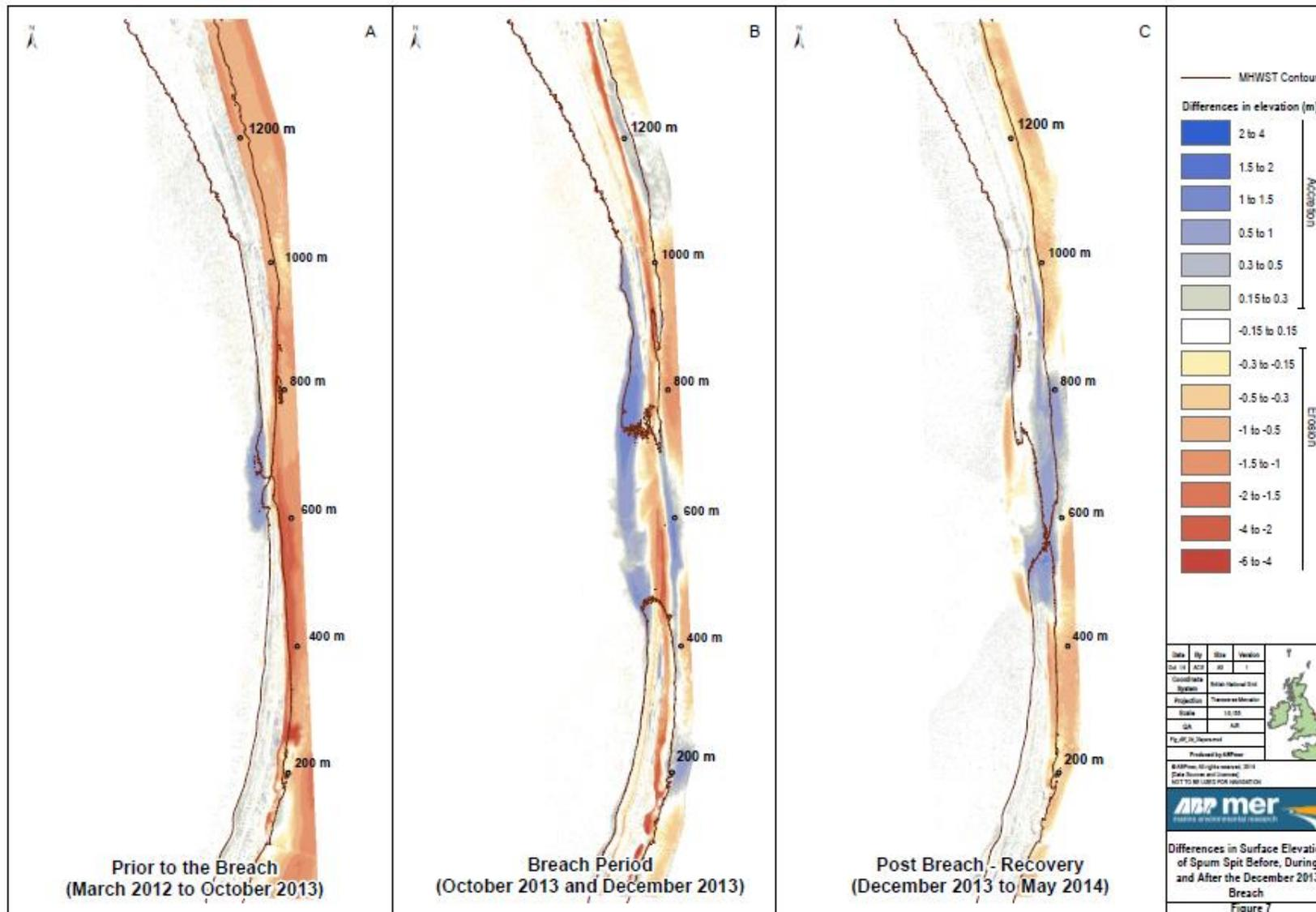
Figure 25 Differences in surface elevation before and after the 2014 temporary breach (from ABP mer 2014)
