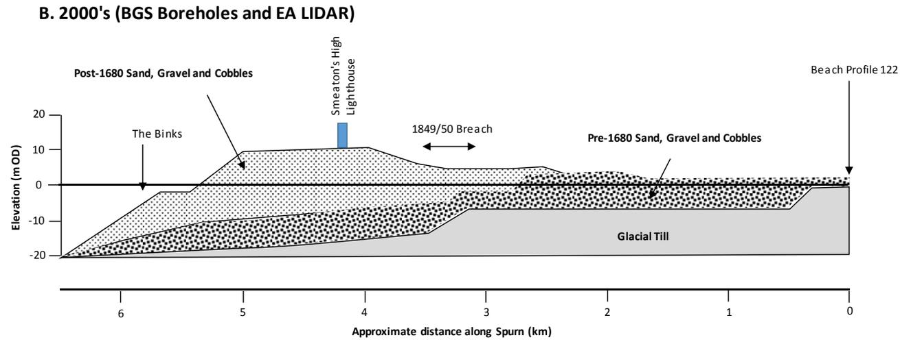
Figure 40 A schematic model showing how Spurn has changed since the late 17<sup>th</sup> Century (the section follows a line down the centre of the present day Spurn. Note the vertical exaggeration)
