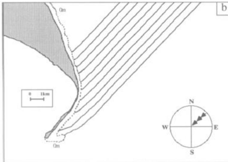
**Figure 4** Wave refraction for NE waves (period 4.25s, height 0.85m). Note that there is little change in wave crest orientation for waves arriving at the Neck, but at the tip waves are refracted towards E (from Ciavola 1997)
