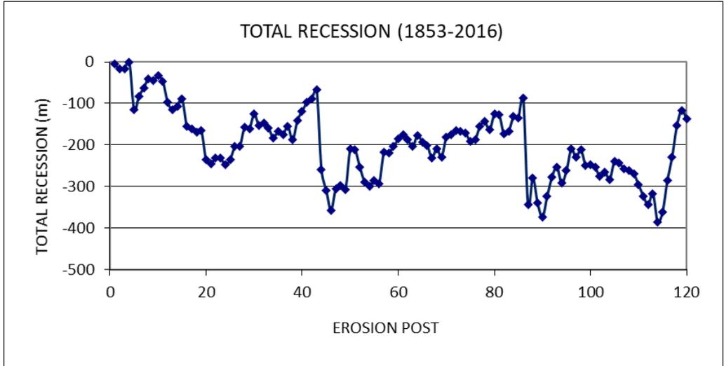
Figure 51 Holderness cliffs: total cliff recession at Erosion Post (EP) locations, 1853-2016 (combined data series)
