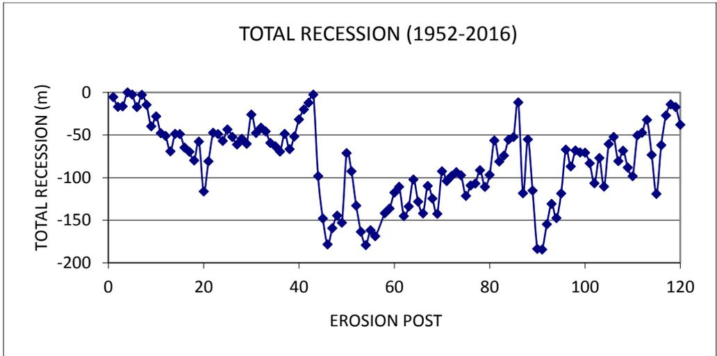
Figure 50 Holderness cliffs: total cliff recession at Erosion Post (EP) locations, 1952-2016 (data for the period 2010-2016 are from the nearest beach profile location)
