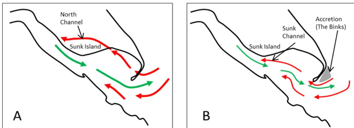
**Figure 48 Flood and ebb channels in the outer Humber (A) Pre-reclamation - early flood enters at Old Den, thence through North Channel (B) Post-reclamation- early flood migrates south allowing accretion of the Binks and elongation of the spit**
