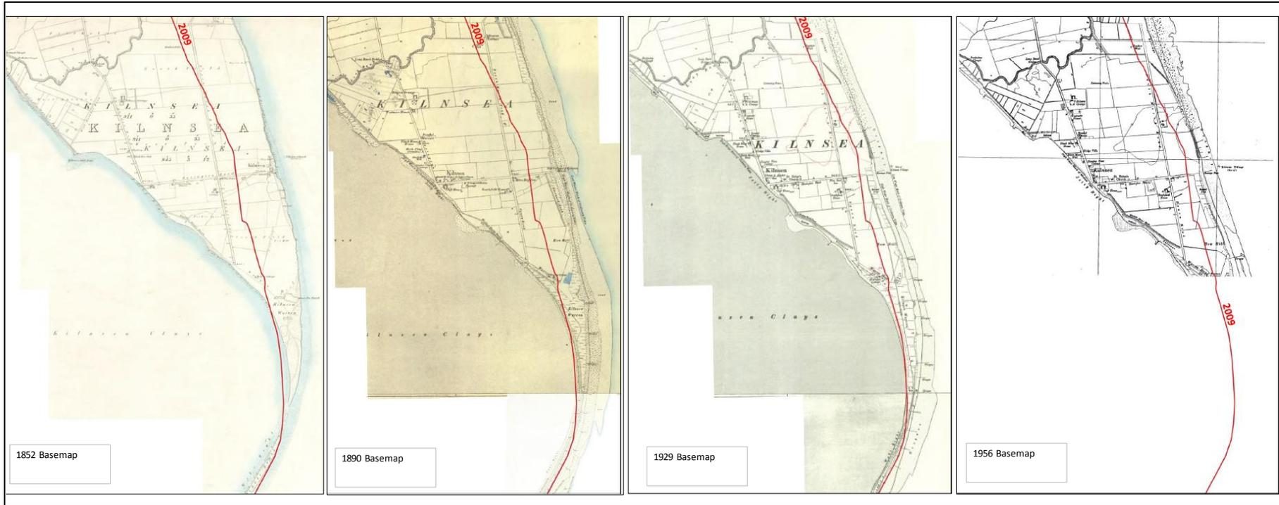
**Figure 43 Comparison of the 2009 Kilnsea-Easington cliffline and Spurn Neck with the positions on earlier Ordnance Survey maps (from L-R: 1852, 1890, 1929, 1956). From Pye and Blott (undated)**
