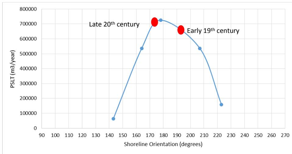
**Figure 39** An indication of the effect of changing shoreline orientation on potential longshore sediment transport (PLST) along the Neck (note that the rates should be seen as relative rather than absolute values). Based on Dalrymple's sediment transport calculator, using 0.5m high NE waves.
