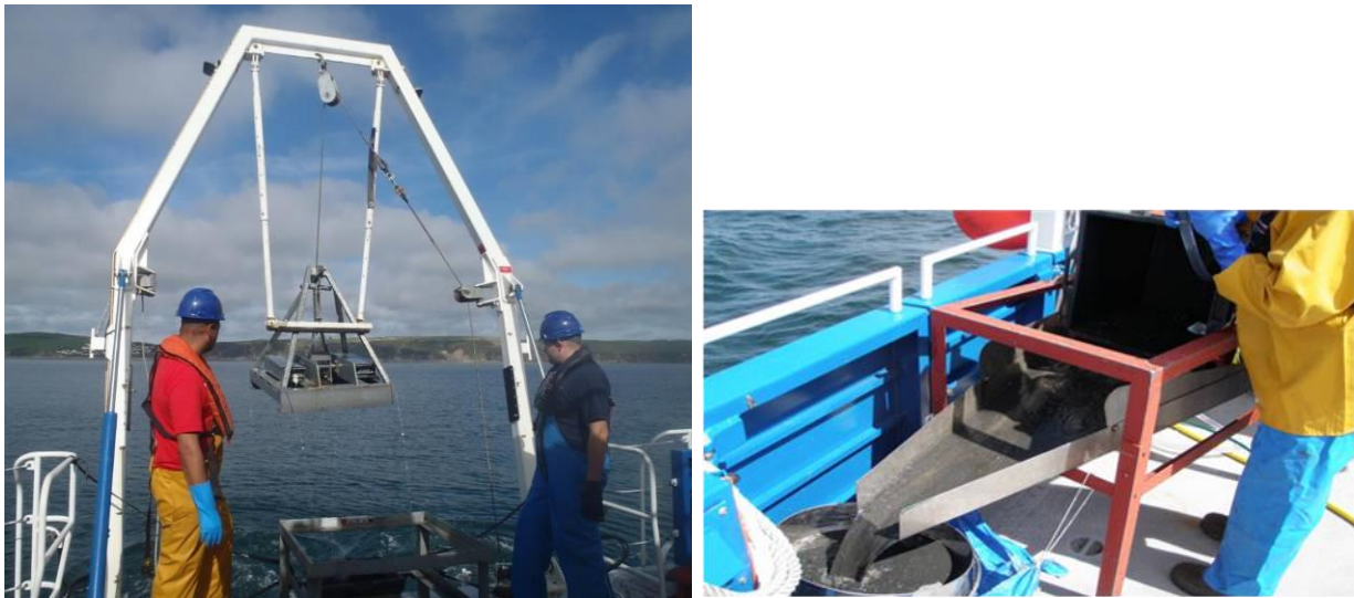
Figure 6. Mini-Hamon grab (left), and equipment for sieving benthic fauna samples (right)
