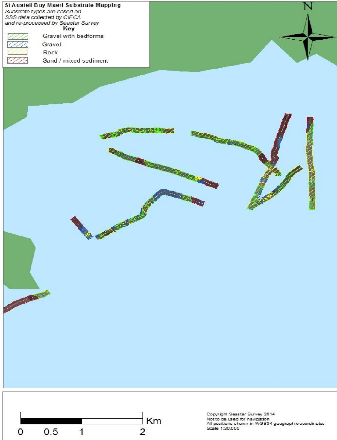
Figure 3.11: Map showing the mapping of the substrate types from the interpretation of the sidescan sonar data.
