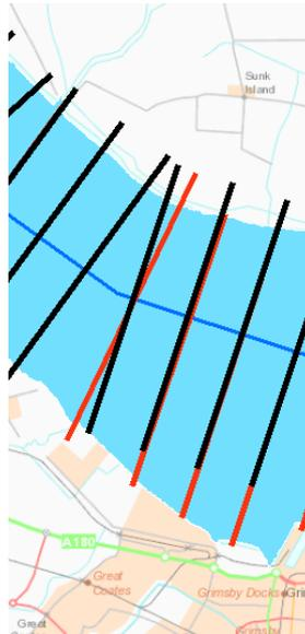
12. Shorten the section lines which cross back onto the estuary; section lines can cross outside the MHWS location
