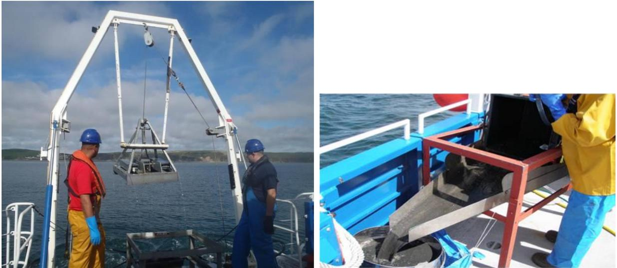
**Figure 9. Mini-Hamon Grab (left), and equipment for sieving benthic fauna samples (right)**
