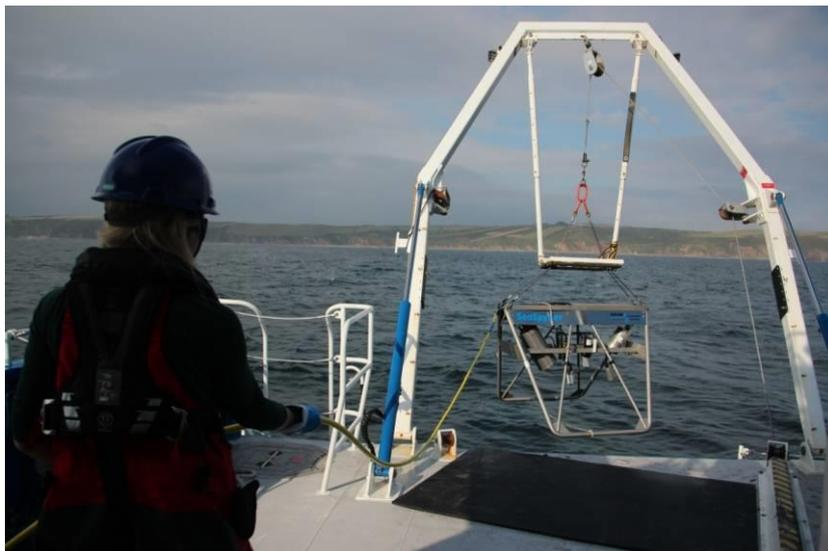
**Figure 8. STR SeaSpyder drop camera system being deployed from the stern of the coastal survey vessel.**
