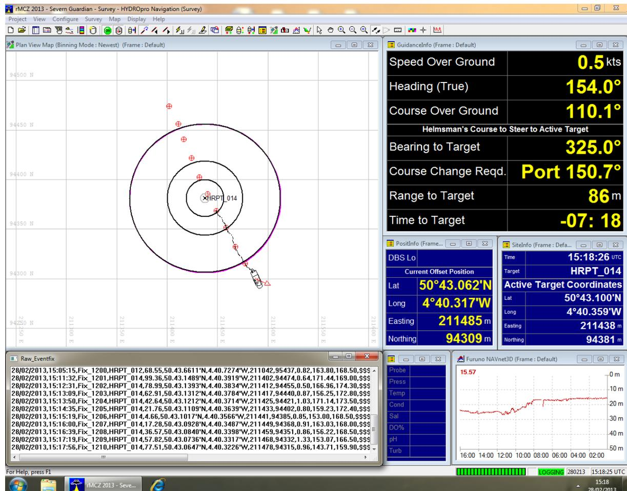
Trimble® HYDRO<sup>pro</sup>™ software screen grab displaying real-time navigation and survey data acquisition for a MCZ drop camera survey line.
