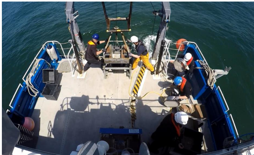
Figure 4. Mini-Hamon Grab and equipment for sieving benthic fauna samples.
