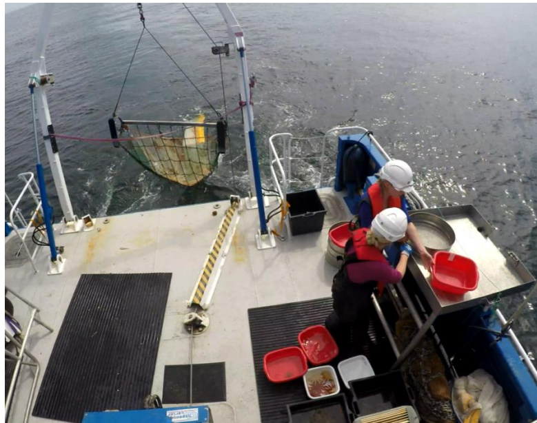
Figure 6. Recovery of the scientific (Jennings) 2 m beam trawl and sample processing on the back deck of the Solent Guardian .
