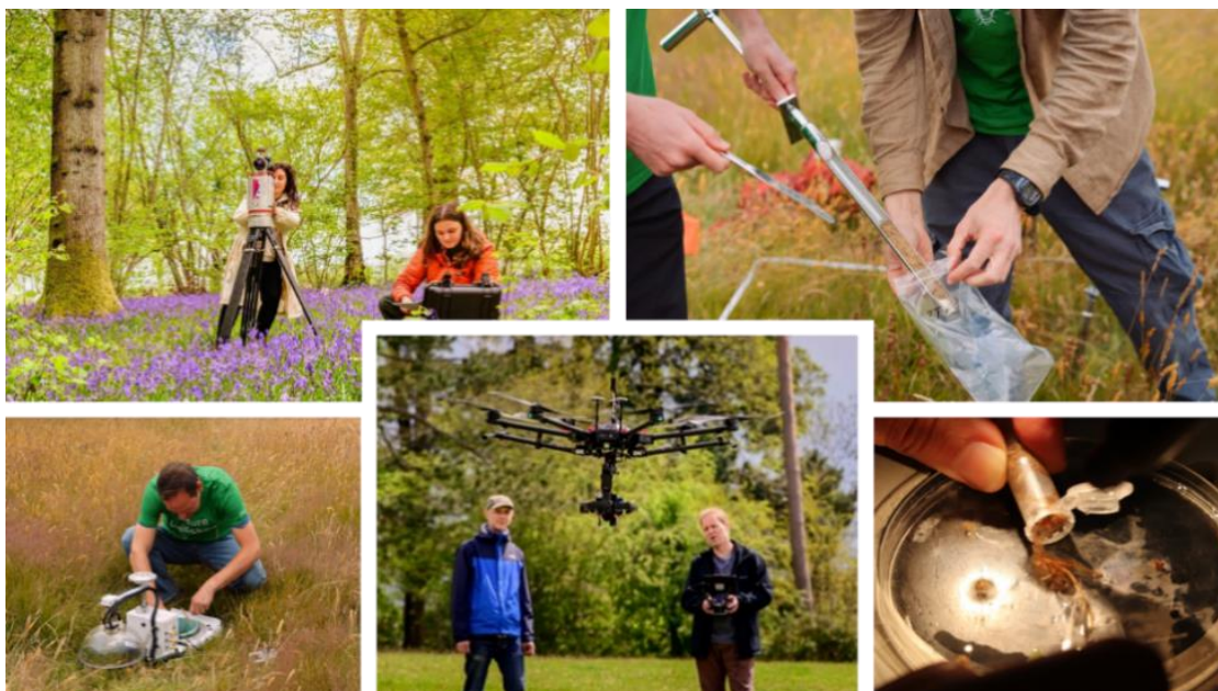
Fieldwork and data collection methods. Top left, clockwise: terrestrial LiDAR scanning of coppice woodland, soil sampling in meadows, root selection and DNA analysis in the laboratory, drone surveys, and gas flux stations in meadows. Photo credit RBG Kew
