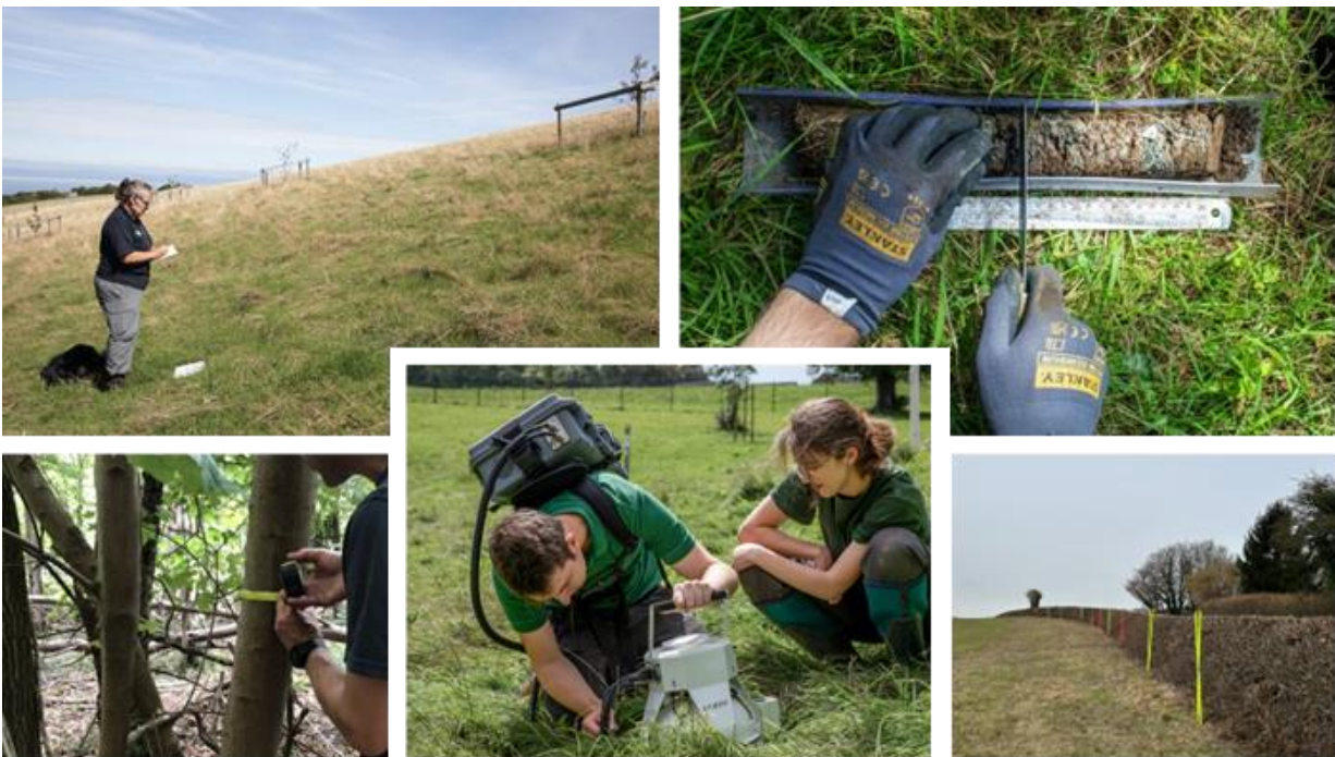
Field data collection methods for carbon science. Top left, clockwise: Species composition and structure of vegetation, soil carbon at 0-15 and 15-30 cm depth, carbon in trees, estimated using measurements of tree height and diameter of stems, carbon dioxide and methane flux from vegetation canopies and soils and carbon in hedgerows and scrub using LiDAR method developed with Kew. Photo credit from top left clockwise: Tamsin Lockwood, Celia Jennings, Tamsin Lockwood, Celia Jennings, Becky Davess
