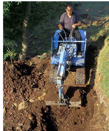
Mini-digger creating a trench at Tideswell Dale, in The Wye Valley SSSI, Derbyshire. The trench exposed the previously hidden lower contact of the Tideswell Dale Sill with the Carboniferous Limestone, increasing understanding of the nature of this igneous intrusion. ©Natural England/Mick Murphy
