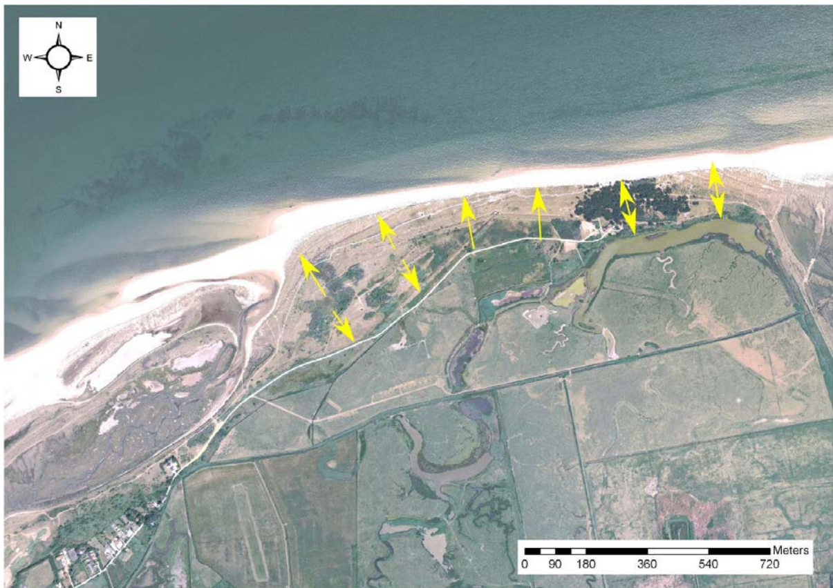
Figure 5. Holme Dunes NNR conceptual groundwater flow diagram. The yellow arrows indicate the likely direction of groundwater flow. © NERC (CEH) 2013. © Next Perspectives.
