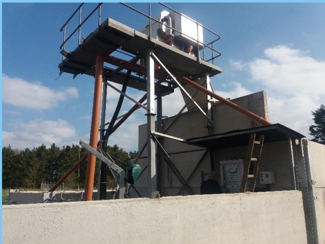
The Sperrin Optiflow slurry separator at Portway Farm is a key component in the new slurry handling system, managing slurry from 310 high-yielding Holstein cows housed on sand bedded cubicles.
