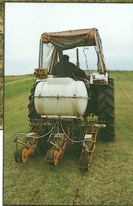
Stanhay precision slot-seeder with a bandspray attachment. Seedlings were more vigorous and survived better in the longer term. (Photo: Groundwork Trust)
