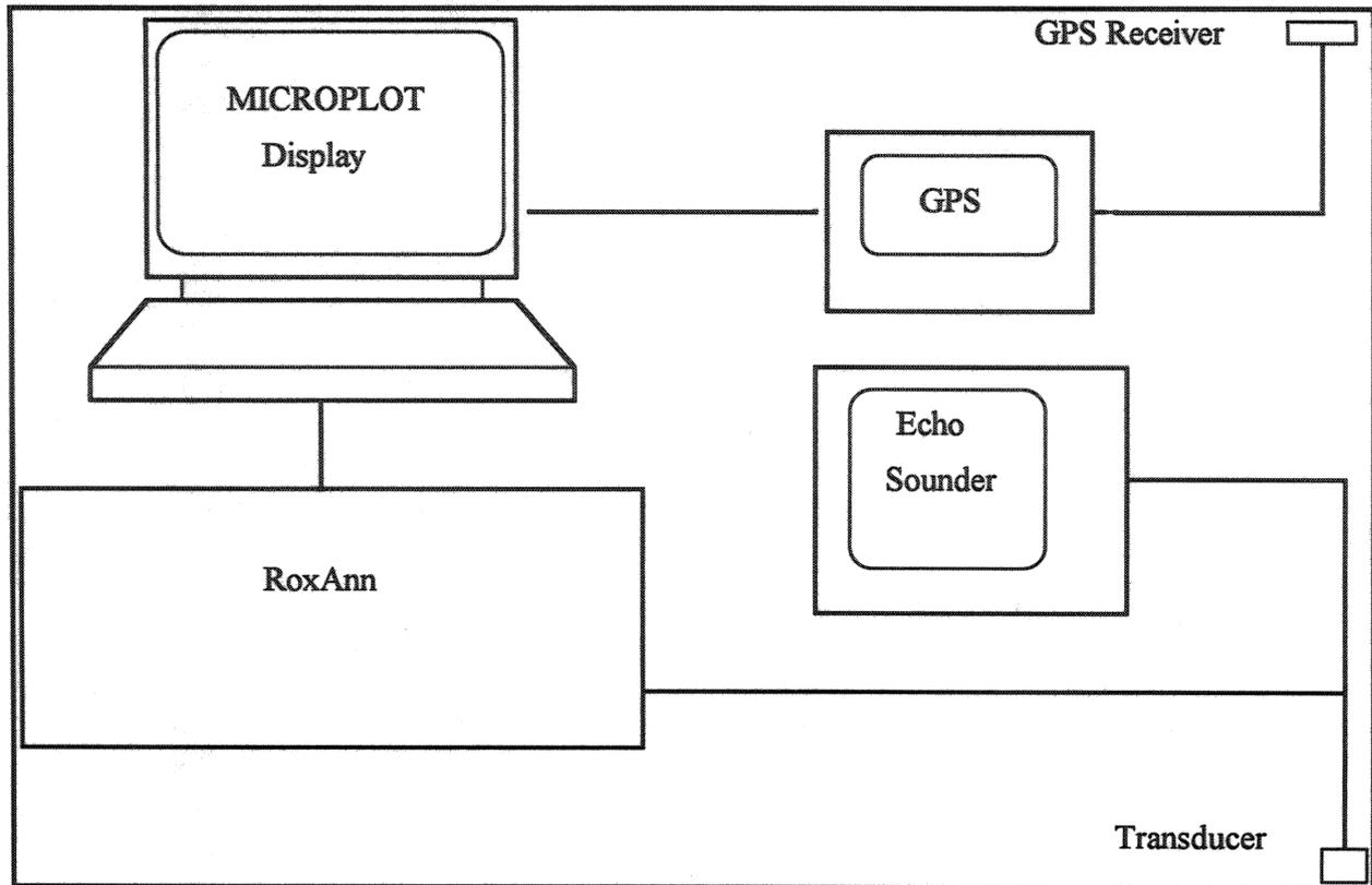
**Figure 2 Schematic diagram of acoustic survey equipment**
