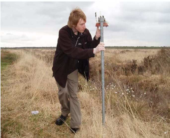
Measuring ammonia using passive diffusion tubes at Fenn's and Whixall Moss in Shropshire (courtesy of Dr Joan Daniels)
