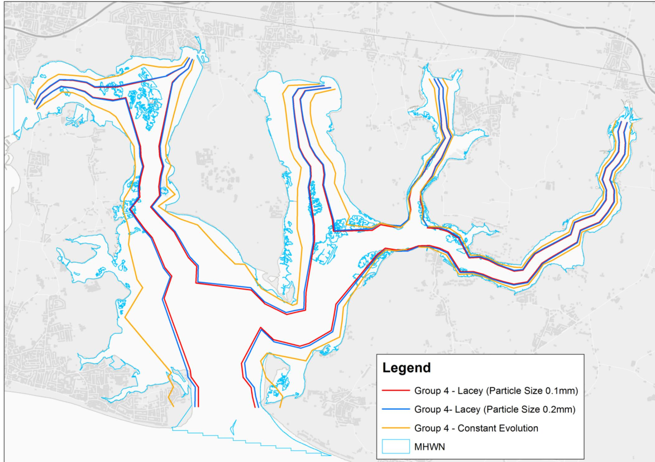
Figure 5.6. Comparison of observed and predicted widths in Chichester Harbour using the regime equation for United Kingdom estuaries Group 4 combined with 1. particle size of 0.1mm in the Lacey (1930) equation (red), 2. particle size of 0.2mm in the Lacey (1930) equation (blue), and 3. the 'constant evolution' relationship (orange)
