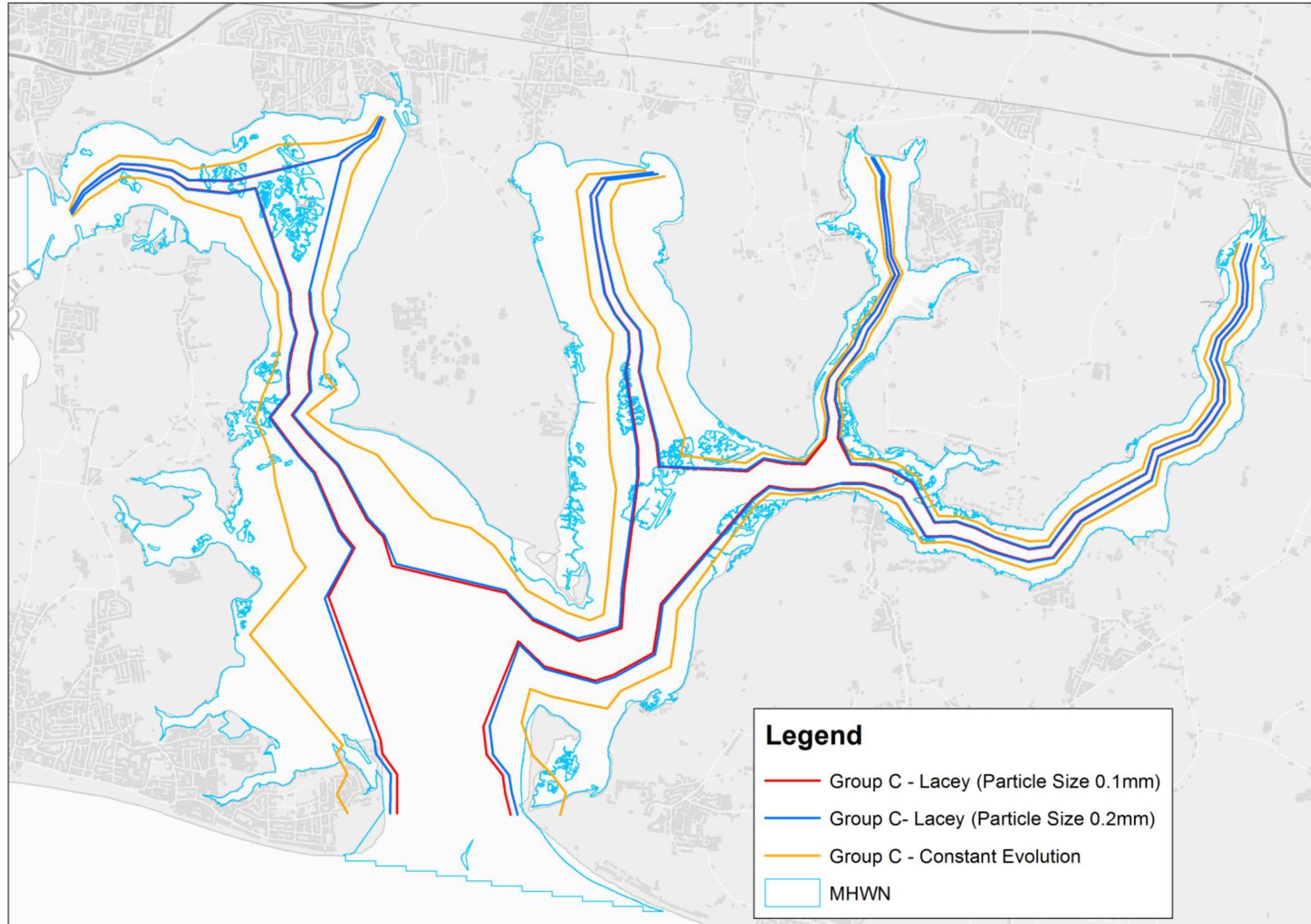
Figure 5.5. Comparison of observed and predicted widths in Chichester Harbour using the regime equation for United Kingdom estuaries Group C combined with 1. particle size of 0.1mm in the Lacey (1930) equation (red), 2. particle size of 0.2mm in the Lacey (1930) equation (blue), and 3. the 'constant evolution' relationship (orange)
