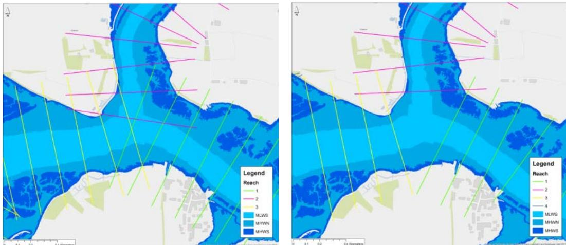
**Figure 4.9. Example of when to manually move or remove automated sections that overlap at channel confluences**
