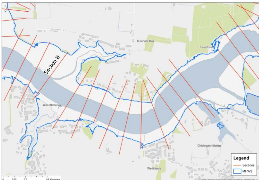
**Figure 4.8. Examples of when to manually remove automated sections that cut across both the main channel and a tributary channel**
