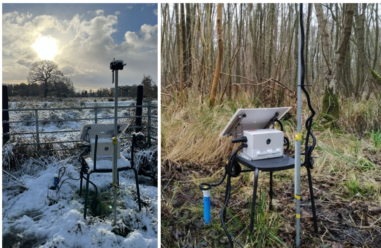
Figure 3-2 Photographs of peat cameras in situ (credit: John Spill, left photo, and Jonay Jovani, right photo © UKCEH)
