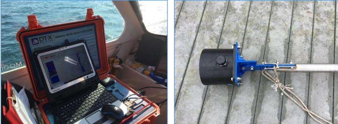
**Figure 3.** The BioSonics DT-X Extreme surface unit (left) and pole-mounted 200 kHz transducer (right).
