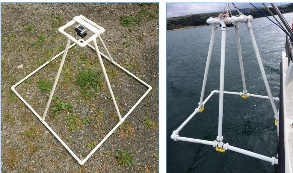
**Figure 2.** The 1 m<sup>2</sup> photo-quadrat with GoPro camera mounted directly above the quadrat
