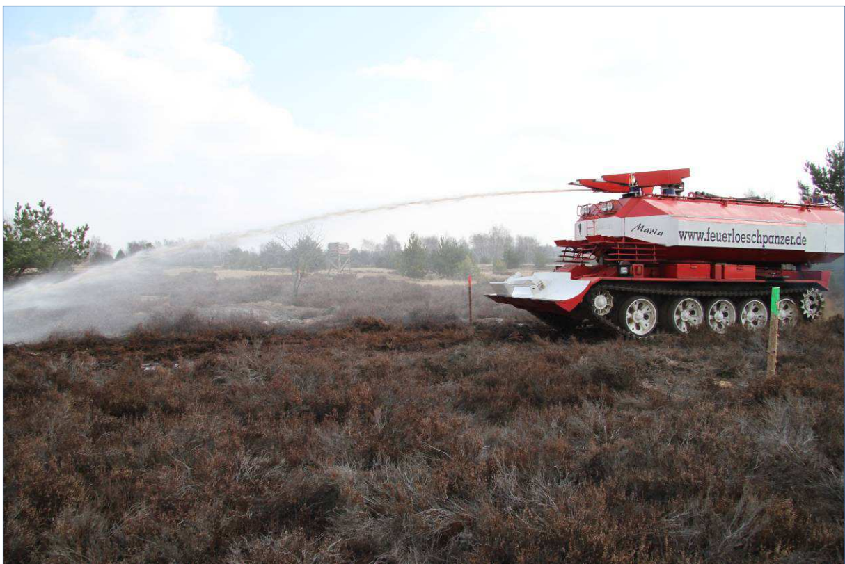
A specially tailored tank for employment in the prescribed burning of heathlands contaminated with ammunition.
