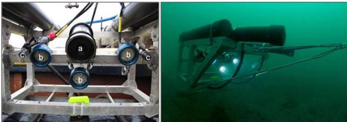
Figure 0.1 Flying array used for the towed video survey. a = high definition video camera, b = LED lights, c = lasers.
