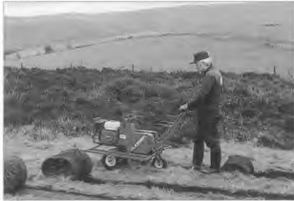
Classen SC-18 Sod cutter
