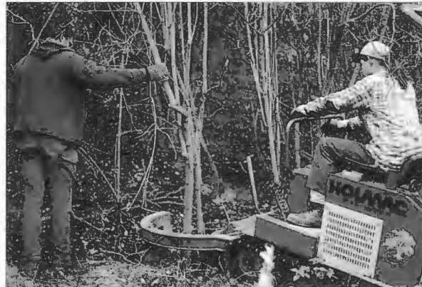
Holmac Root-balling machine
