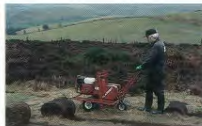
J. Bacon Classen Sod cutter
