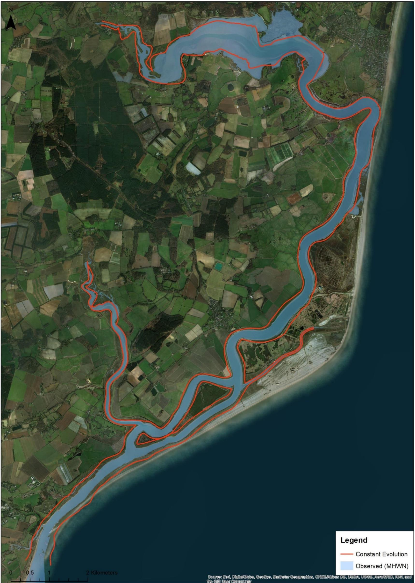
Figure 2.9. Comparison of predicted equilibrium widths with observed widths in the Alde-Ore Estuary (aerial photograph background)
