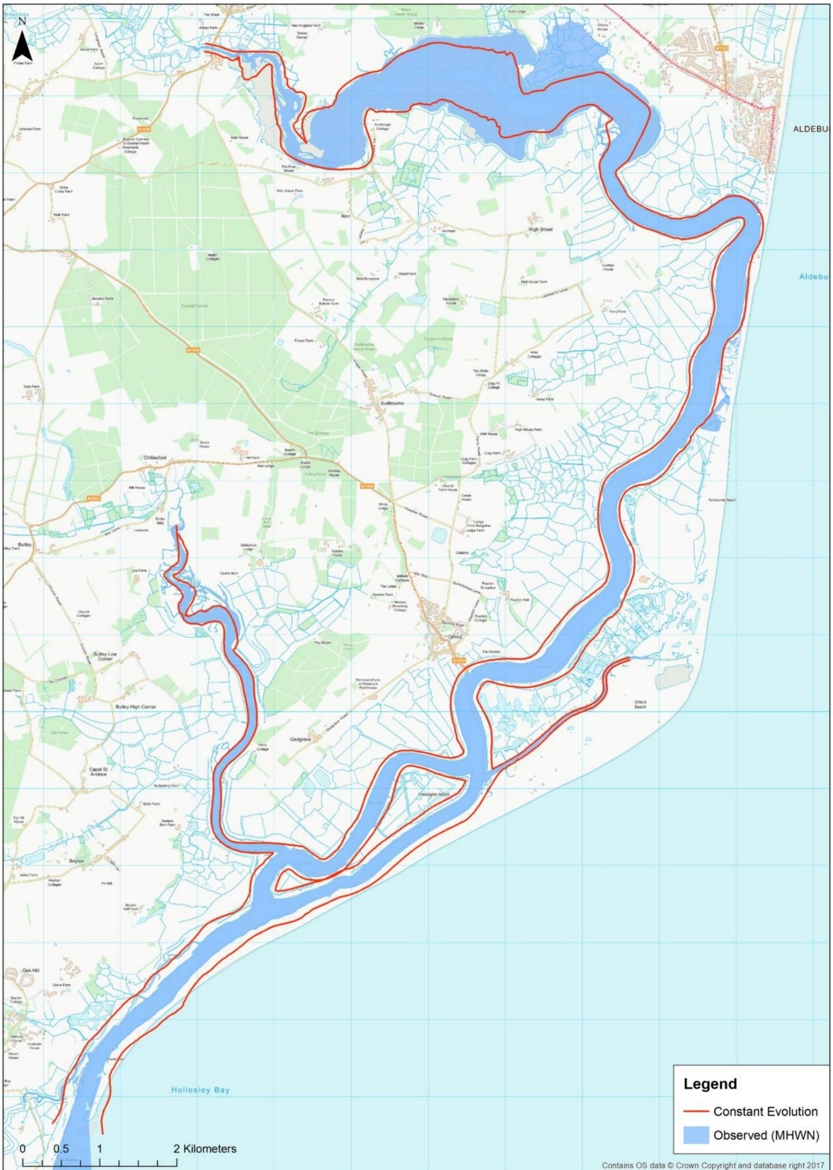
Figure 2.8. Comparison of predicted equilibrium widths with observed widths in the Alde-Ore Estuary (map background)
