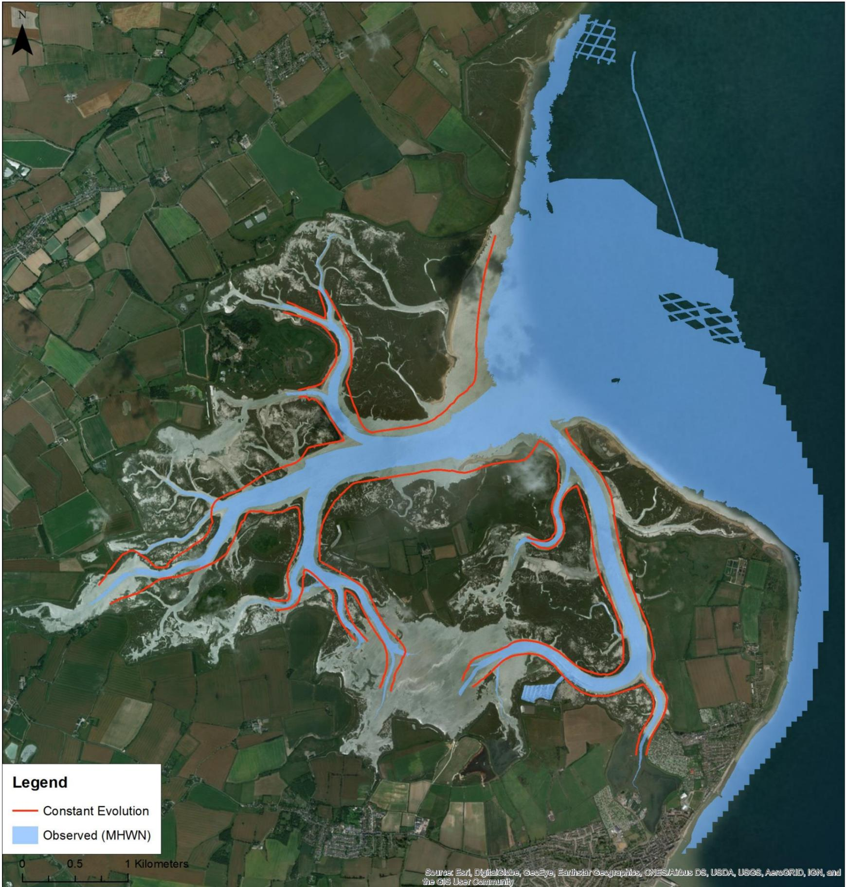
Figure 4.10. Comparison of predicted equilibrium widths with observed widths in Hamford Water (aerial photograph background)
